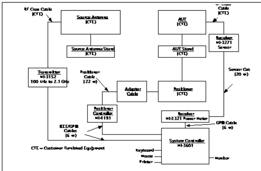
Figure 1. Wiring diagram for typical MI-3610 Antenna Amplitude Measurement System.
