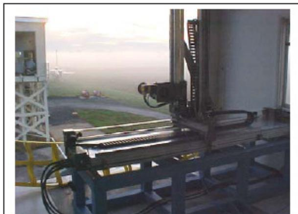
**Fig.2, 5 ft x 5 ft XY Scanner**
