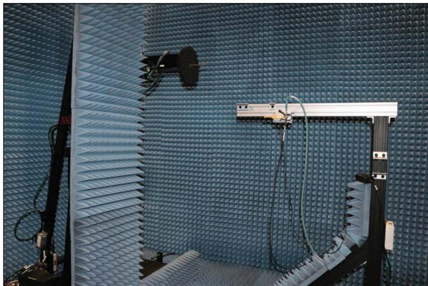
Figure 2: A planar near-field system. Used for measuring highly directive antennas, the electric field is measured in the near-field and a mathematical transform is used to obtain the far field radiation pattern. (photo courtesy of NSI-MI).
