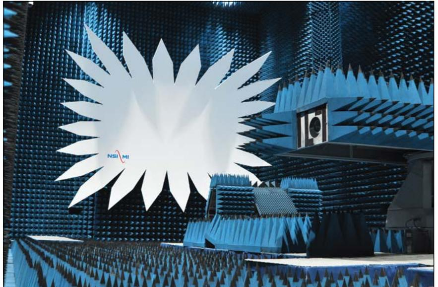
Figure 3: A CATR for testing base station antennas for cellular communications. (photo courtesy of NSI-MI)
