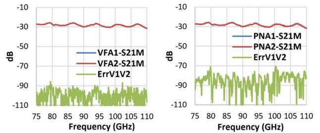
Figure 2. Transmission repeatability for DUT1: VFA and PNA
