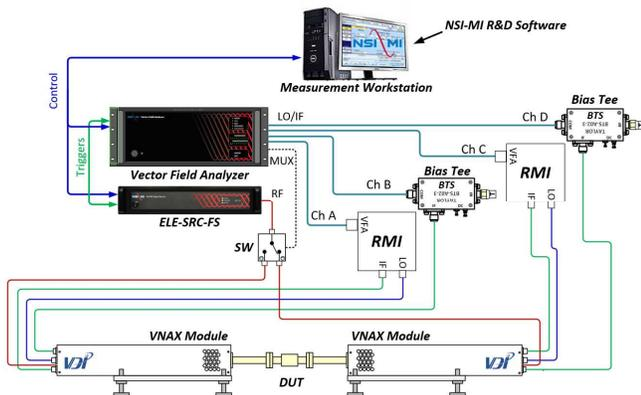
Figure 1. NSI-MI VFA setup with VDI VNAX modules
