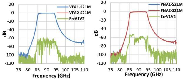
Figure 4. Transmission repeatability for DUT2: VFA and PNA
