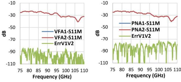
Figure 3. Reflection repeatability for DUT1: VFA and PNA
