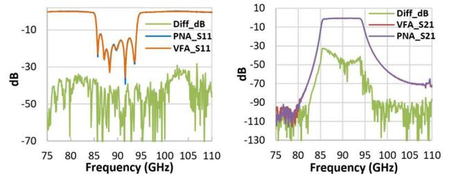
Figure 13. Measurement comparison for DUT2: S11 and S21
