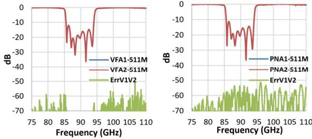
Figure 5. Reflection repeatability for DUT2: VFA and PNA
