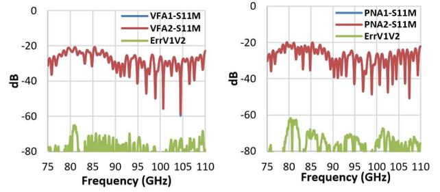
Figure 7. Reflection repeatability for DUT3: VFA and PNA
