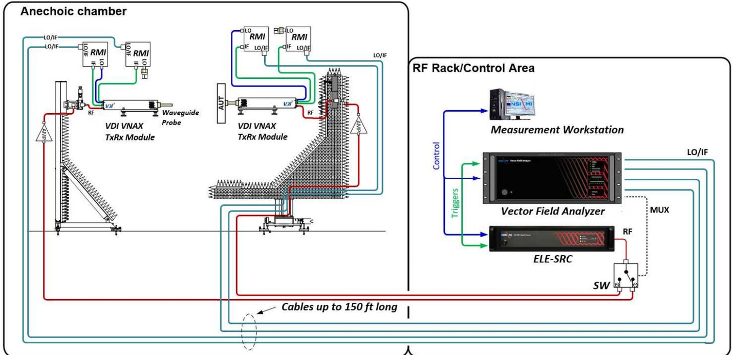
Figure 15. Example of a VFA based antenna measurement system
