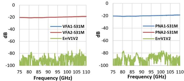
Figure 6. Transmission repeatability for DUT3: VFA and PNA
