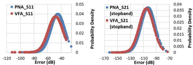
Figure 10. Error distribution for DUT2: S11 and S21
