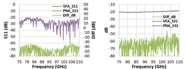
Figure 14. Measurement comparison for DUT3: S11 and S31
