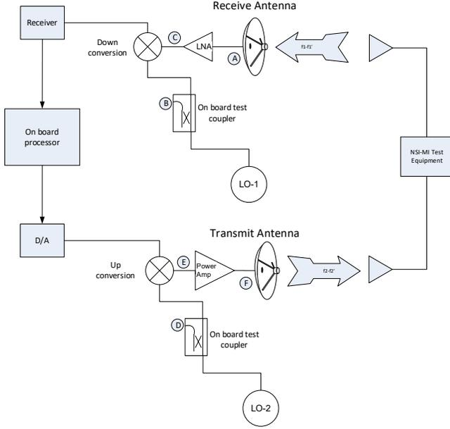
Figure 1. Notional payload system block diagram
