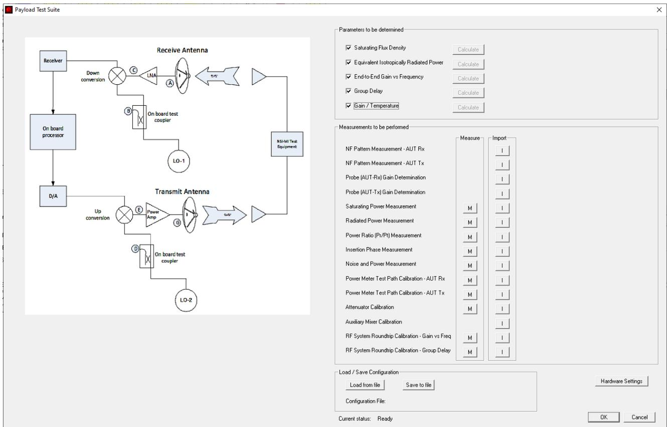
Figure 6. Payload Test Suite (PTS) software GUI
