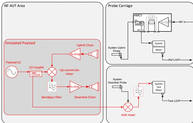
Figure 2. Block diagram of the simulated payload and RF test system
