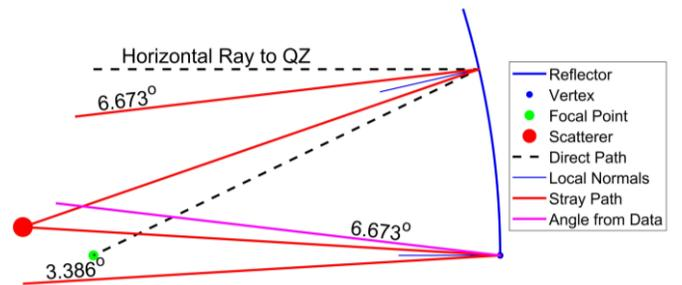
Figure 3 Geometry with scatterer behind focal plane.
