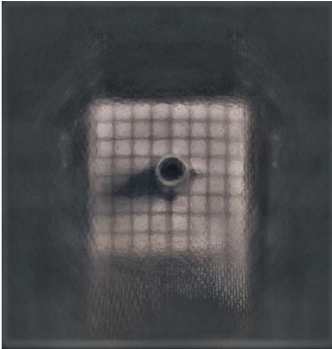
Figure 1 Photo of paper-target grid just behind feed through polished rolled-edge reflector.
