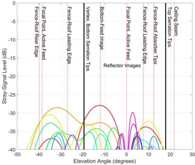
Figure 5 Final stray-signal mapping.
