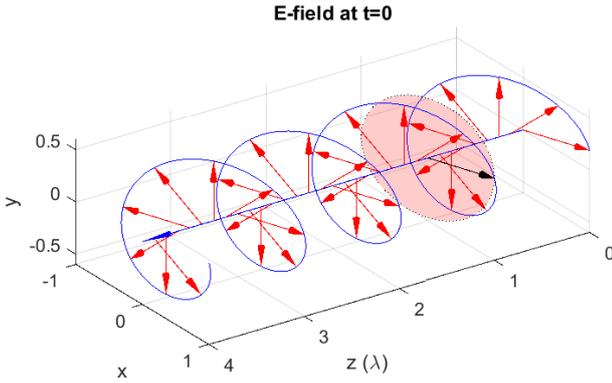
Figure 2. 3-dimensional wave representation for  $E_1 = 1$  and  $E_2 = 0.6e^{j(0.4\pi)}$  at time  $t=0$
