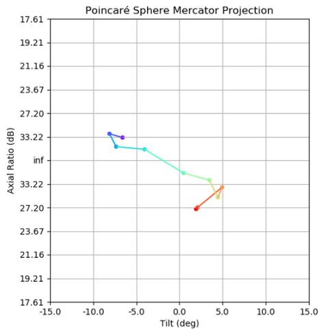
Figure 6. Poincaré sphere plot with Mercator projection using elliptical parameters showing polarization state vs frequency for a measured antenna (top: full-scale, bottom: zoomed in)
