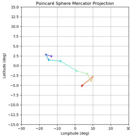
Figure 4. Poincaré sphere plot with Mercator projection showing polarization state vs frequency for a measured antenna (top: full-scale, bottom: zoomed in)
