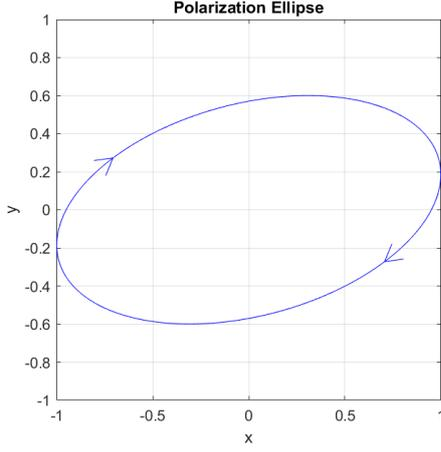
Figure 1. Polarization ellipse associated with  $E_1 = 1$  and  $E_2 = 0.6e^{j(0.4\pi)}$
