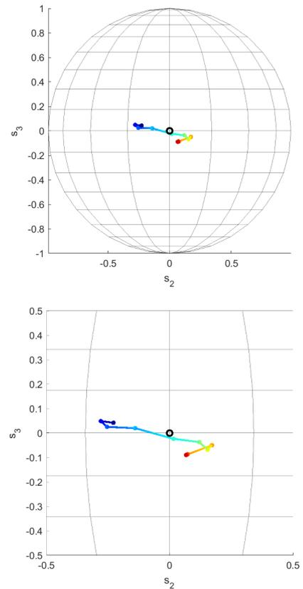
Figure 3. Poincaré sphere plot showing polarization state vs frequency for a measured antenna (top: full-scale, bottom: zoomed in)
