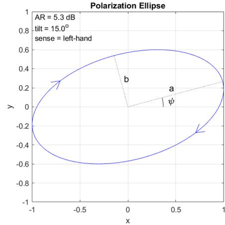
Figure 5. Polarization ellipse associated with  $E_1 = 1$  and  $E_2 = 0.6e^{j(0.4\pi)}$  with graphical and textual annotations
