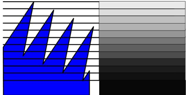
**Figure 3. The tilted pyramid at “low frequencies” becomes a series of layers of effective permittivity that fail to provide any improvement and may be detrimental.**
