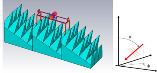
**Figure 6. Model of the tilted absorber showing the angles of arrival.**
