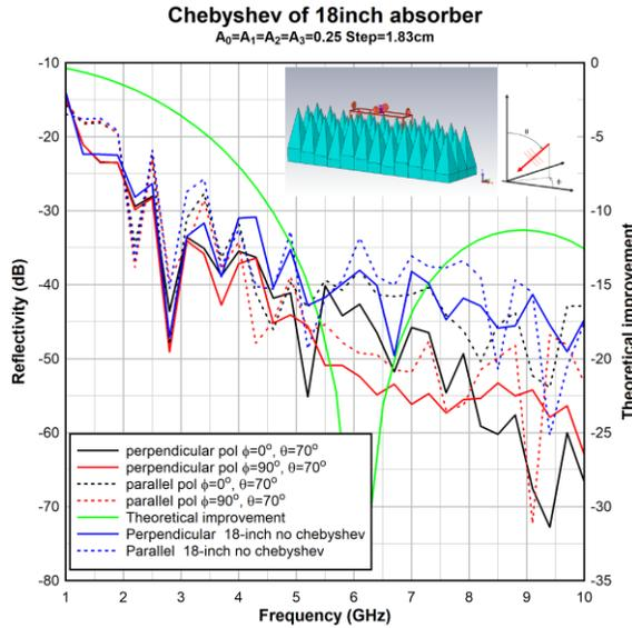
**Figure 5. Results for the bi-static reflectivity for standard 18-inch, and a Chebyshev absorber arrangement across and along the propagation direction.**
