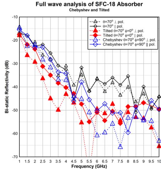
**Figure 7. Results for the tilted absorber reflectivity at  $70^\circ$  of incidence compared to the standard 18-inch absorber and to the Chebyshev.**
