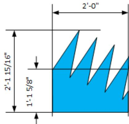
**Figure 4. 18-inch typical pyramidal absorber tilted 22°**
