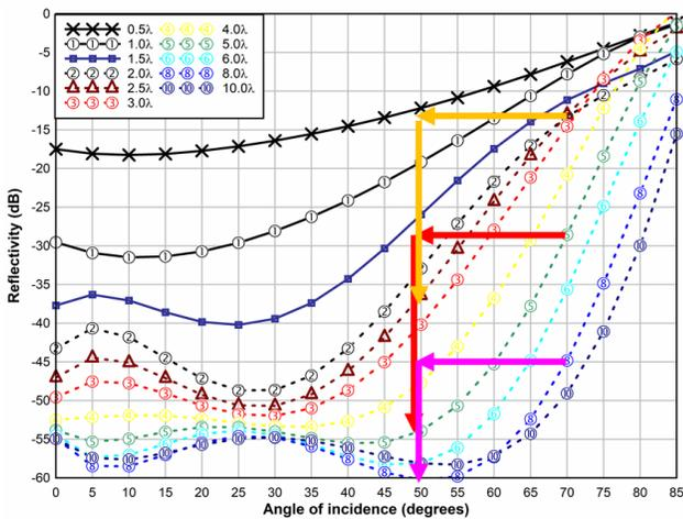
**Figure 2. Bi-static reflectivity of RF absorber versus angle of incidence for different electrical sizes of RF Absorber. Showing the performance improvement by reducing the angle of incidence by 20°.**
