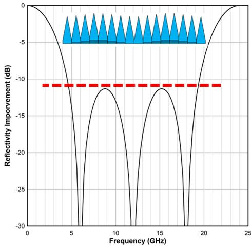
**Figure 1. Theoretical improvement of a Chebyshev arrangement with a 1.83 cm step and equal weights for an angle of incidence of 70° off normal incidence.**
