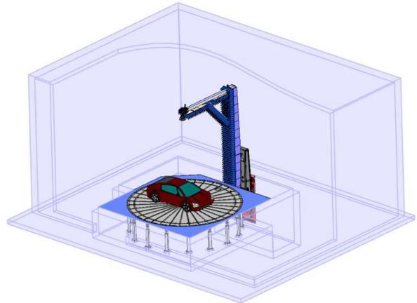
Figure 2. Rendering of Automotive SNF Test System with Stowable Gantry
