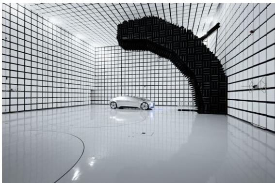
Figure 1. Automotive Test System with High-Accuracy Arch for SNF Measurements and Three Independent Turntables. Photo Courtesy of Frankonia Germany EMC Solutions GmbH
