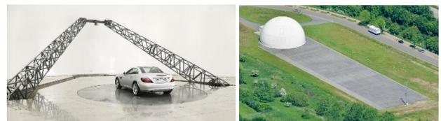
Figure 3. ATC Antenna Test Range in Itzehoe, Germany with Views of the SNF System inside a Radome (left) and Outdoor Far-Field Range (right)
