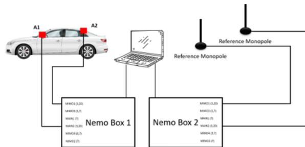
Figure 5. LTE Band 20 2x2 MIMO Drive Test Setup
