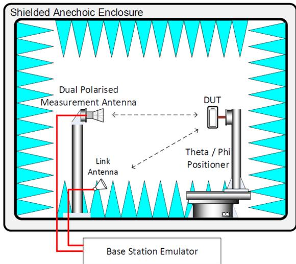
Figure 4. OTA Test Setup
