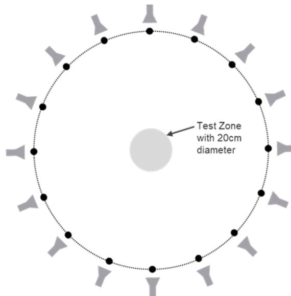
Figure 7. Multi-Probe Anechoic Chamber (MPAC) Diagram from 3GPP Standards showing Array Configuration for 20 cm Quiet Zone
