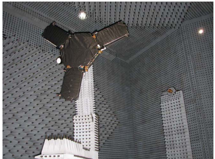
Figure 3. DTU-ESA Spherical Near-Field Antenna Test Facility. Calibration of “MIROS” radiometer.
