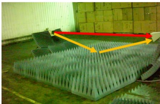
Fig. 1. Absorber reflectivity measurement at large angles of incidence
