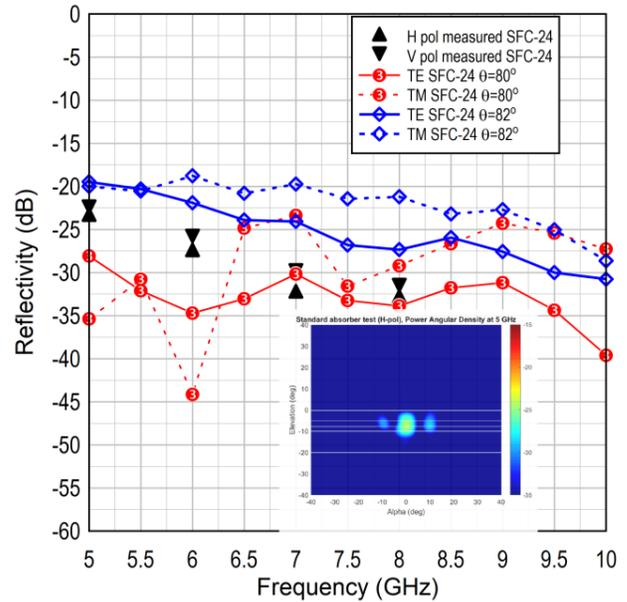
Fig 3. Measured and computed results for SFC-24 showing good agreement between them. The inset shows the measurement results at 5 GHz.
