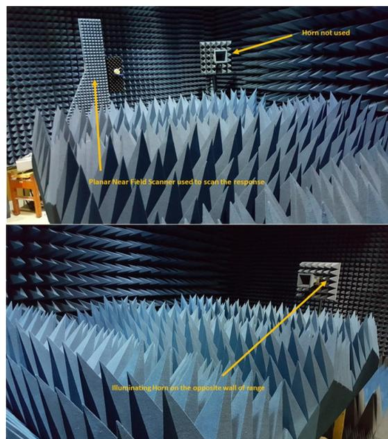
Fig. 2. Measurement set up, receive side (top) and transmit side (bottom)
