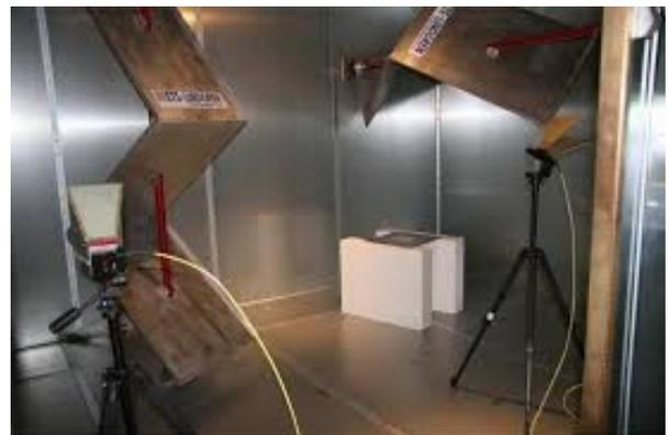
Figure 3. Interior of a reverberation chamber
