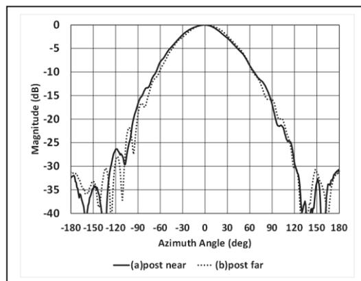
Figure 2. 2.4 GHz Radiation pattern under differing test conditions
