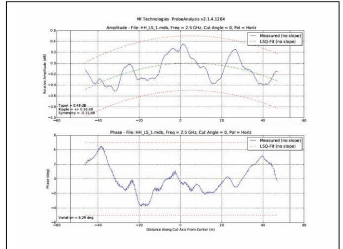
Figure 5. Horizontal field probe cut made at horizontal polarization
