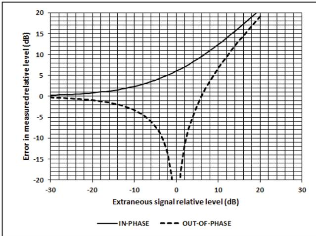
Figure 3. Possible error in measured relative pattern level due to extraneous signals[2]
