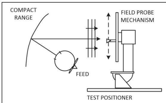
Figure 4. Field Probe Configuration
