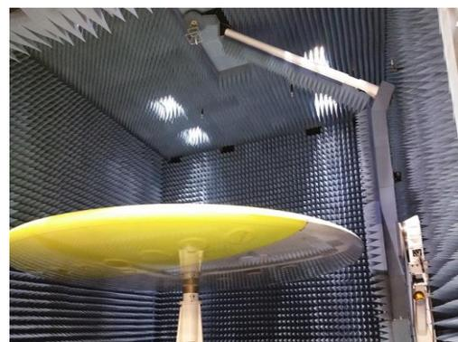
Figure 4. US Navy  $\theta/\phi$  SNF system with very large AUT
