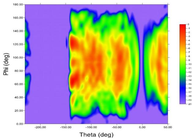
Fig. 9. Far-field transformation from Near-Field measurement with radial correction
