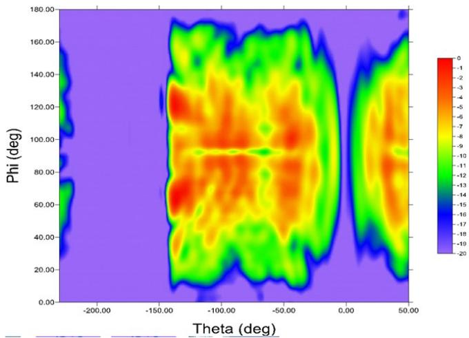
Fig. 8. Far-field transformation from Near-Field measurement without radial correction
