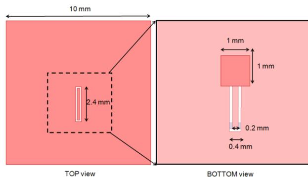
Fig. 4. Antenna dimensions
