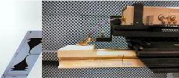
Figure 5. UT Dallas AUT probe platform with orientation of planar antenna.
