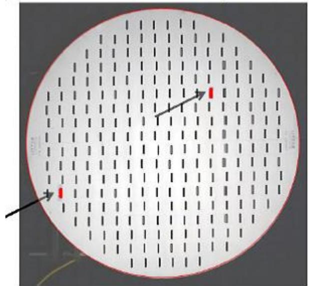
Figure 3: Overlay of Element Map and Photograph of the 45.7 cm (18 in) Flat Plate Array
