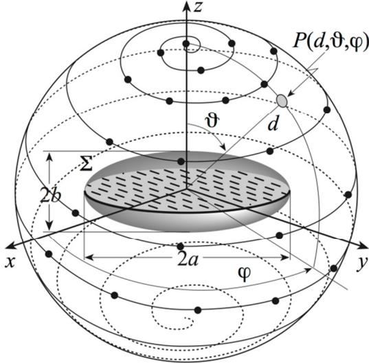
Figure 2: Spherical spiral scanning for a quasi-planar AUT.
