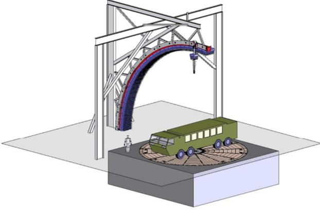
Figure 1: A SNF system for measuring antennas mounted on large vehicles.
