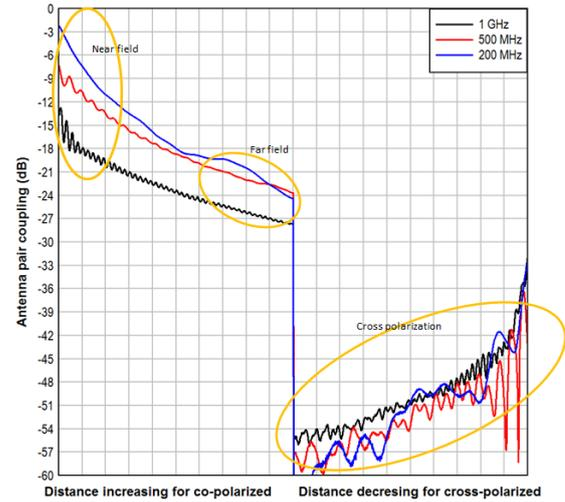
Fig. 6. Antenna pair coupling at different frequencies versus distance for the co-polarized and cross-polarized scans measured in an extrapolation range. The distance is not shown on the x-axis, but the maximum distance of separation in the range is 10m. The plot is given as a typical sample of the data that is gathered during the sample
