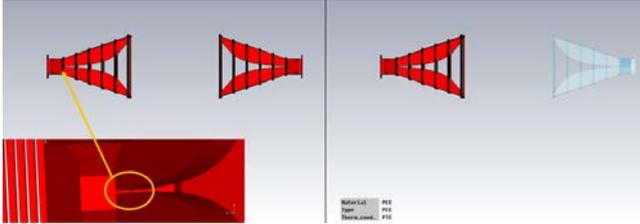
Fig. 2. The two simulations executed. on the left the two antennas present. On the right one simulation with one antenna while the other is modelled as vacuum. in the inset there is picture of the location of the discrete feed.
