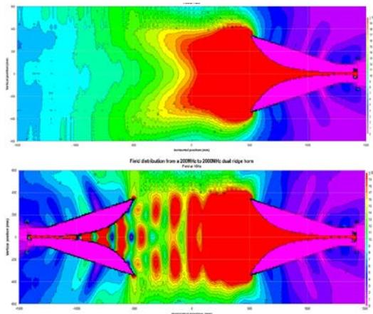
Fig. 4. The electric field distribution shown at 1GHz for the antenna by itself (on the top) and for the antenna in the presence of a secondary unit during the calibration process (on the bottom).
