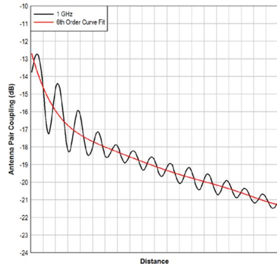
Fig. 7. Polynomial approximation to the measured data in the extrapolation range at 1 GHz.
