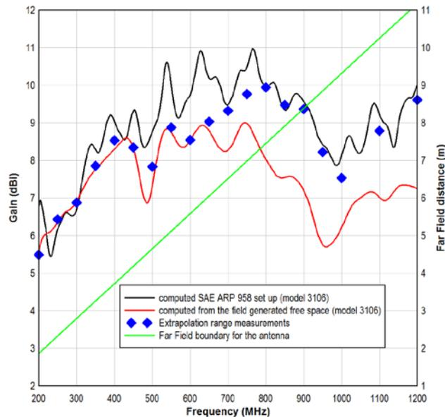
Fig. 8. Comparison of the computed SAE approach and the single antenna gain measurement to the Extrapolation range interpolation measurement.
