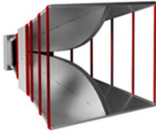
Fig. 1. A Dual Ridged Horn Antenna used in the measurements and the simulations. The antenna aperture is 73cm by 93cm with a 97cm length
