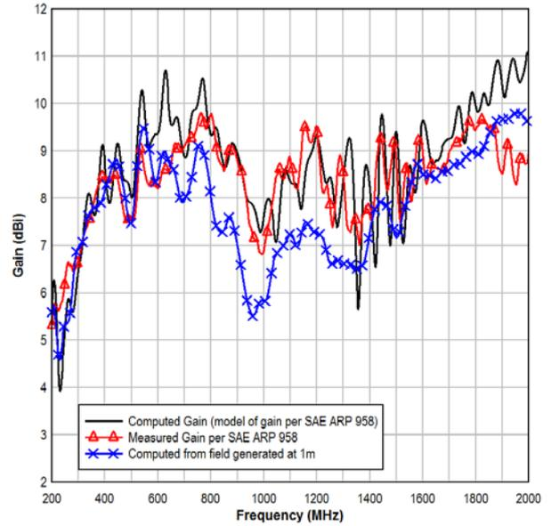
Fig. 3. Numerical results and measurements of the gain of a dual ridge horn covering the range from 200 to 2000 MHz at 1 m distance.
