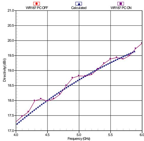
Figure 3. WR187 Standard Gain Horn Measured with WR187 OEWG Probe showing Negligible Effect of Probe Pattern Correction on Directivity
