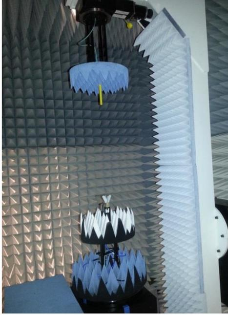
Figure 5. Characterizing the Quad-Ridged Horn on the NSI Spherical Near-Field System
