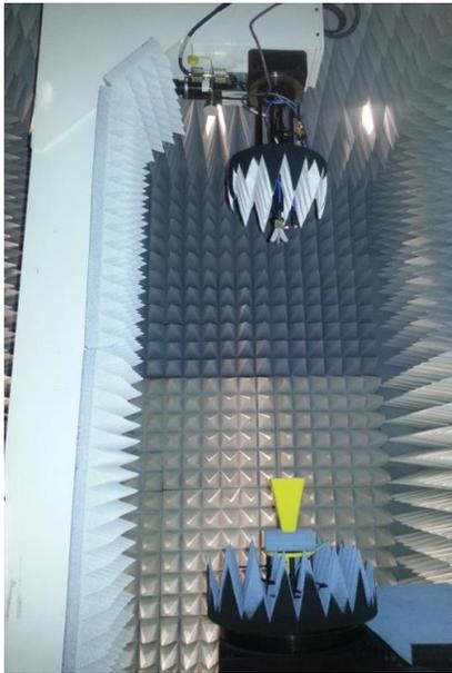
Figure 9. WR28 Standard Gain Horn Antenna Measured using WR28 OEWG Probe on NSI SNF Range
