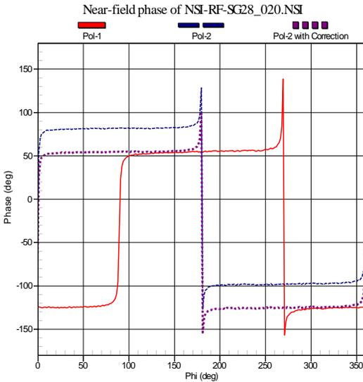
Figure 7 Near-field  $\theta = 0^\circ$  Polarization Cuts before and after  $34^\circ$  Correction Applied to  $\chi = 90^\circ$  Data
