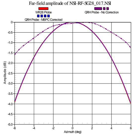
Figure 8. Far-Field E-Plane Cut Main Beam showing Effects of Channel Imbalance and Improvement using MPCB Algorithm
