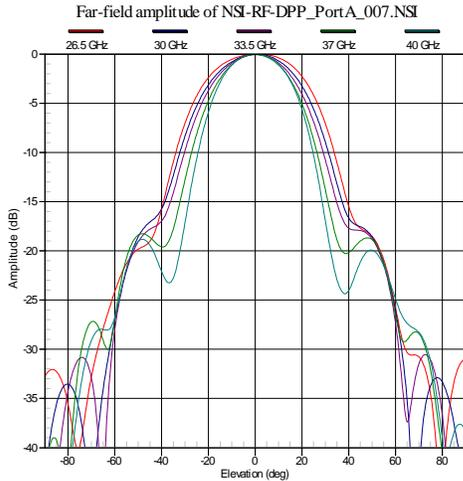
Figure 6. H-Plane Pattern of the QRH's X-Port at Select Frequencies
