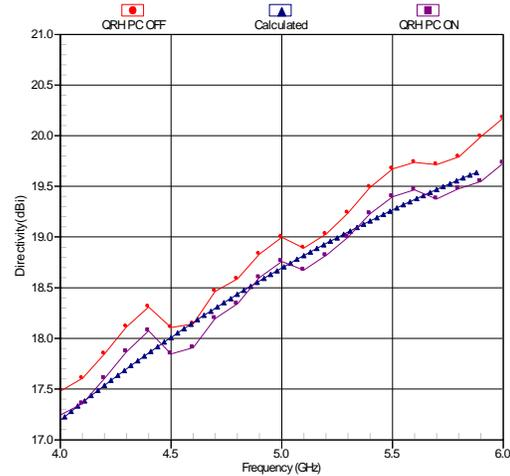
Figure 4. WR187 Standard Gain Horn Measured with DRH Probe showing Impact of Probe Pattern Correction on Measured Directivity
