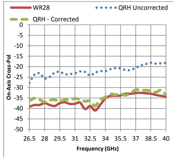
Figure 10 On-Axis Cross-Pol of WR28 Horn Measured with WR28 OEWG and QRH Probe with and without Correction
