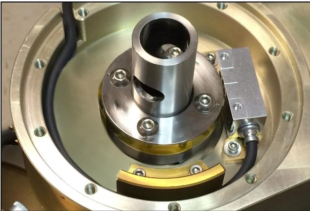
**Figure 3. Direct Drive Encoder Installation**
