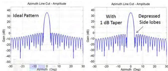
Figure 9. Results of Introducing Amplitude Taper
