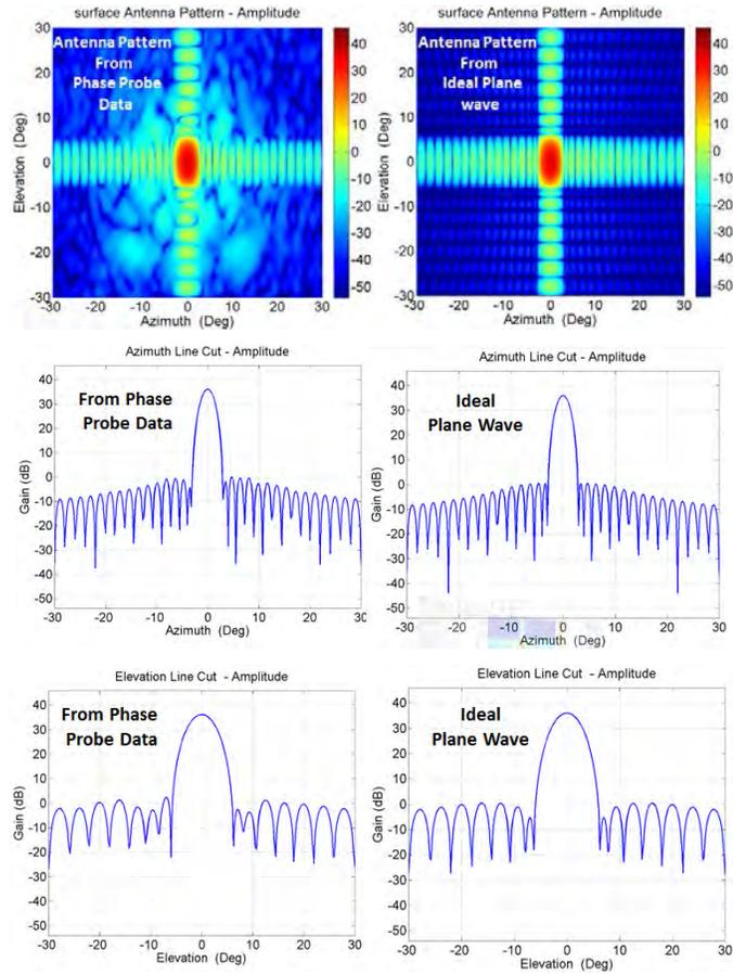
Figure 11. Antenna Pattern Comparison
