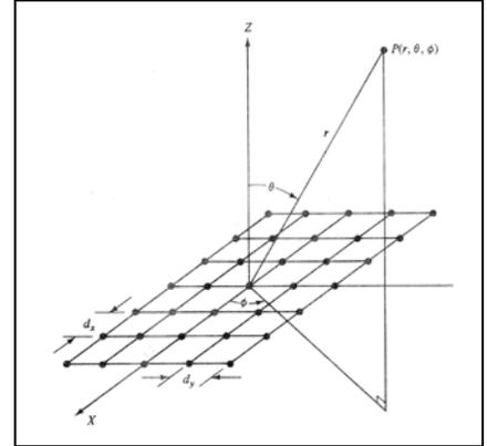
**Figure 2. Planar Array: elements arranged in a Rectangular Grid**
