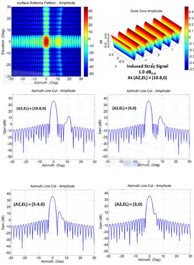
**Figure 6. Walking Stray Signal from off Axis to Main Center**
