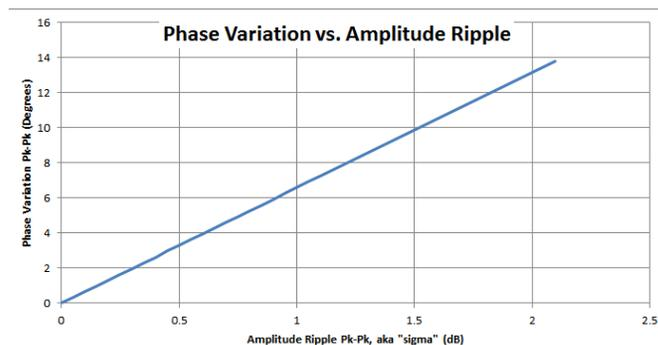
**Figure 5 At small amplitude, Phase Variation  $\Delta$  and Amplitude Ripple  $\sigma$**
