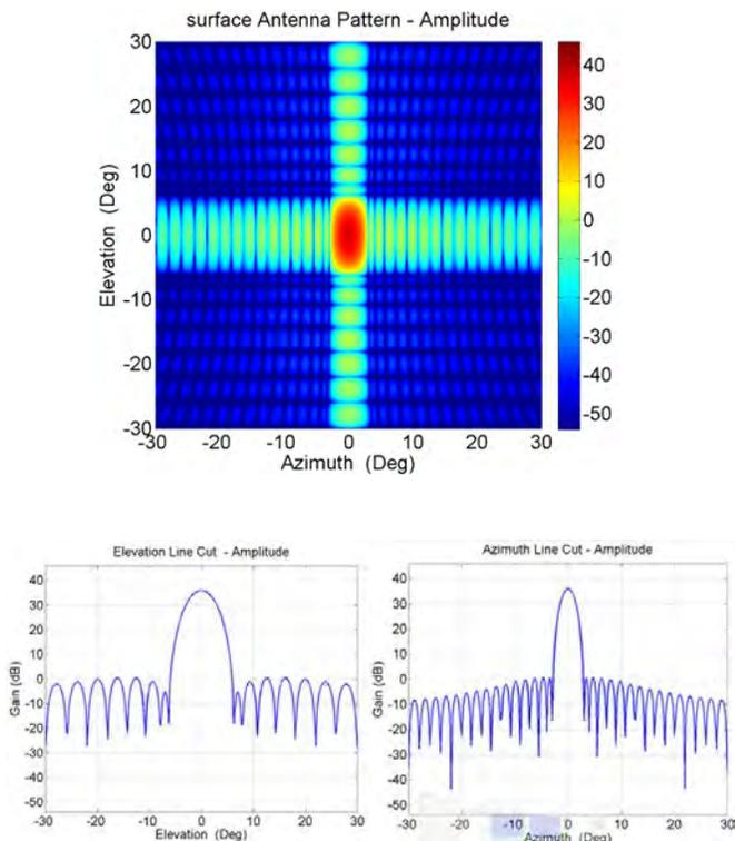
**Figure 3. Equation (5); 2.5 GHz 4 X 2 m array, 35 dB Taylor NBAR=6; perfect QZ**
