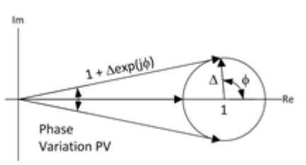
**Figure 4. Relationship between Phase Variation PV & Amplitude Ripple**
