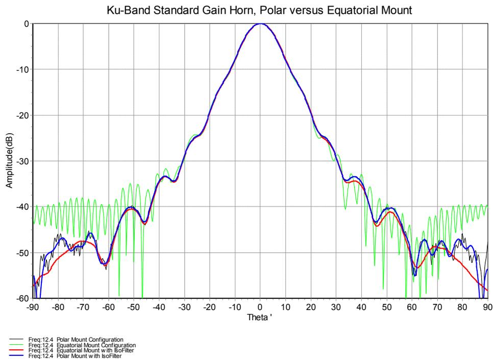
**Figure 4: Comparison Plot of Far-Field H-Plane pattern of the SGH.**
