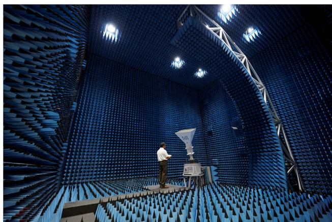
Figure 1 Arch over Azimuth Spherical Near-field Measurement System.
