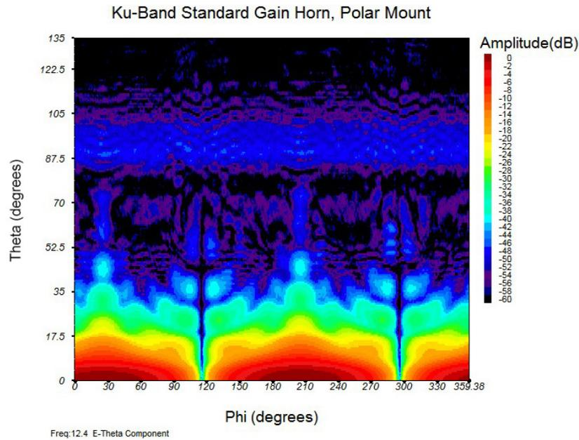
**Figure 3: Contour plot of the E-Theta component of the measured near-field. Note the band of RF leakage between 80 and 120 degrees.**
