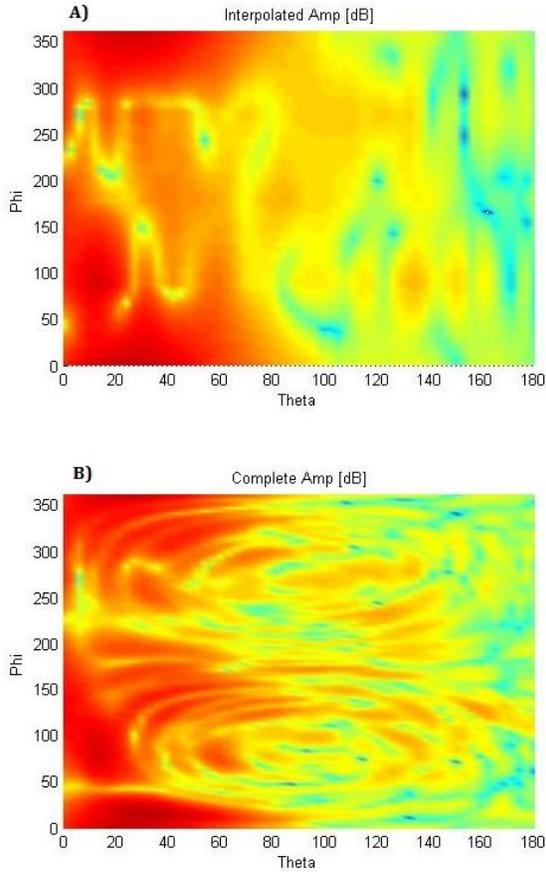
Fig.3: A) Interpolated  $\theta$ -polarized NF amplitude using pre-conditioning Method #1, B) Amplitude of the acquired  $\theta$ -polarized NF for a base station antenna.
