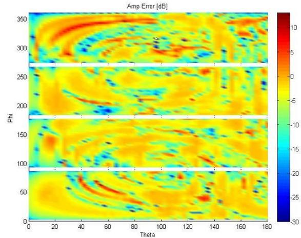
Fig.1: Amplitude error of the pre-conditioned NF data values (over the measurement sphere) using interpolation Method #1 for a base station antenna.
