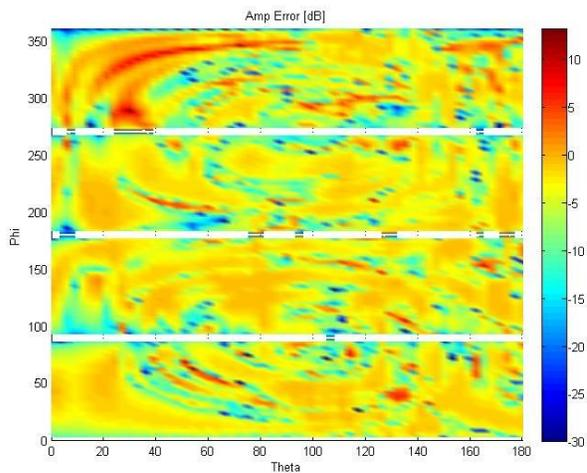
Fig.2: Amplitude error of the pre-conditioned NF data values (over the measurement sphere) using interpolation Method #2 for a base station antenna.
