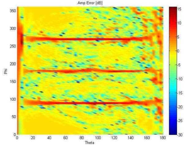
Fig.4: Amplitude error of the pre-conditioned NF data values (over the measurement sphere) using interpolation Method #3 for a base station antenna.
