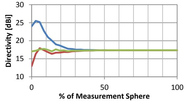
Fig.5: Comparison of acquisition without pre-conditioning (—), with pre-conditioning Method#1 (—), and with pre-conditioning Method#2 (—).
