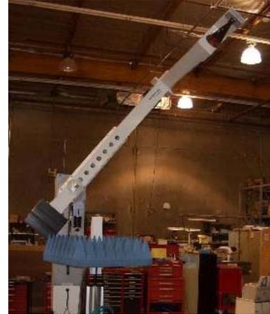
Fig. 1. NSI-RF-WR284 OEWG probe being tested at NSI on NSI-700S-90 in open factory environment with no anechoic chamber.
