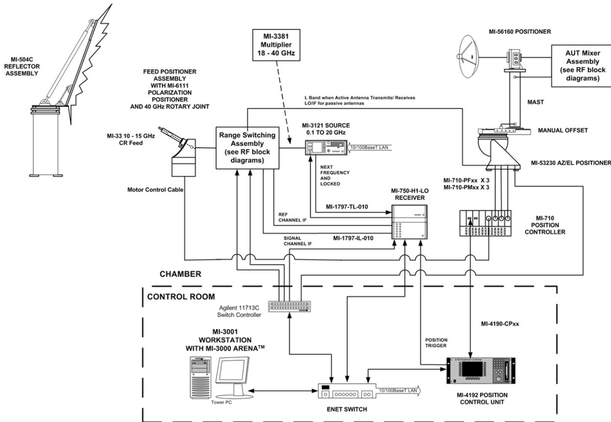
Figure 3 – Overall System Block Diagram
