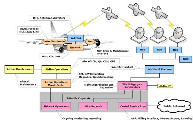
Figure 1 – Typical IFEC Network Architecture [2]
