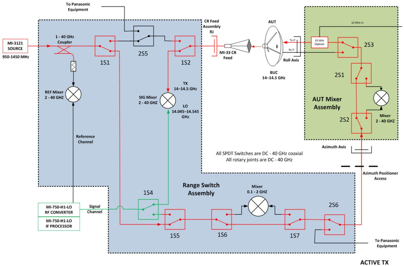
Figure 4 – Range Switching Assembly (Active Tx Mode Shown)
