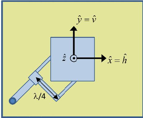
**Figure 1 – Microstrip Patch Antenna**
