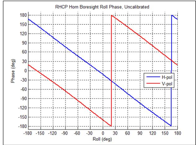
**Figure 3 – Bore-sight Roll Phase for a RH AUT with AR < 0.5 dB**
