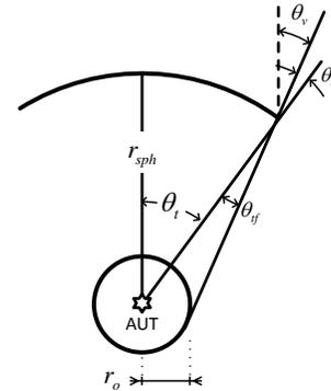
**Figure 1 - Conventional Truncation Geometry of SNF Measurement Sphere**
