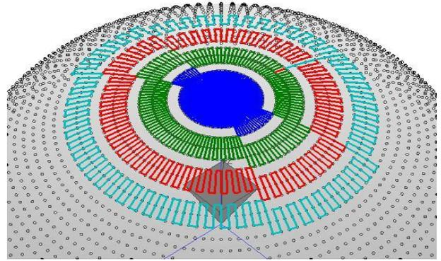
**Figure 3 - Acquisition map obtained using the second acquisition rule considered in the paper, after four iterations. NF points on the measurement sphere are denoted by the  $\circ$  symbols. The acquisition map consists of the set of loci shown, each colour representing those points sampled during a different iteration. A horn AUT is shown at the sphere centre.**
