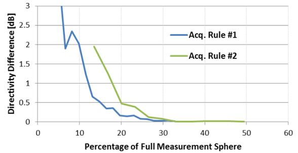
Figure 9 - Evolution of change in directivity for the two different acquisition rules, for the SGH as AUT, as the acquisition map increases.
