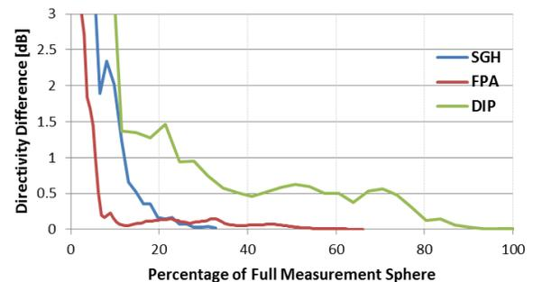
**Figure 5 - Co-polarized directivity difference in the direction of maximum directivity  $(\theta_0, \phi_0)$  for each of the AUTs in Table 1.**
