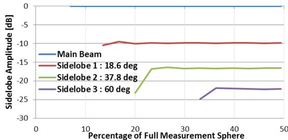
Figure 7 – Amplitude of the highest three sidelobes, relative to the radiation pattern maximum value, for the SGH as AUT.
