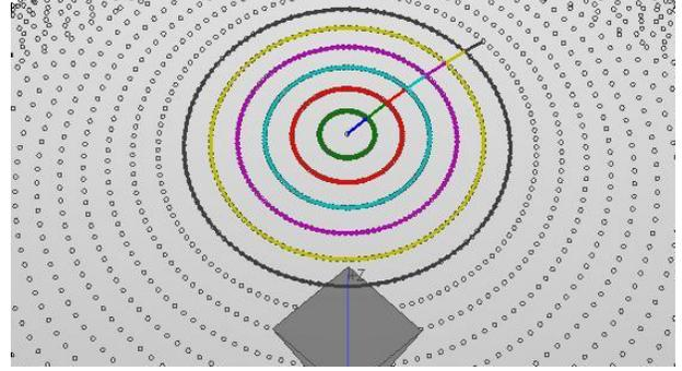
**Figure 2 - Acquisition map obtained using the first acquisition rule considered in the paper, after seven iterations. NF points on the measurement sphere are denoted by the  $\circ$  symbols. The acquisition map is the set of circles shown, each colour representing those points sampled during a different iteration.**
