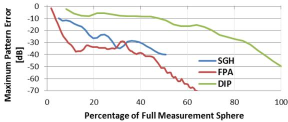
Figure 6 - Normalized co-polarized pattern error in the direction where this error is largest, for each of the AUTs in Table 1.
