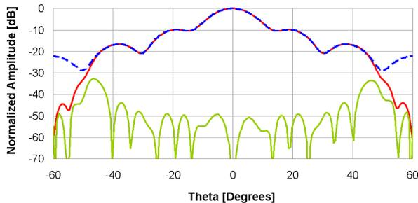
Figure 8 – Co-polarized radiation pattern of the SGH after eight iterations (—) of the adaptive SNF approach with the second acquisition rule, compared to that obtained from a full sphere acquisition (----). The normalized error function is shown as (—).
