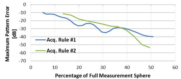
Figure 10 - Evolution of the normalized co-polarized pattern error (in the direction where this error is largest) for the two acquisition rules, with the SGH as AUT, as the acquisition map increases.
