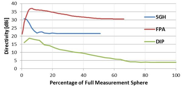
**Figure 4 - Co-polarized directivity in the direction of maximum directivity  $(\theta_0, \phi_0)$  for each of the AUTs.**
