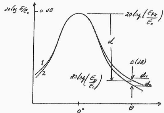
**Figure 1. Two patterns with a discrepancy overlaid. The discrepancy between patterns 1 and 2 at angle  $\theta$  is considered to be due to an apparent stray signal  $E_x$  which adds in phase with  $E_d$  to produce level  $E_1$ , and out of phase with  $E_d$  to produce level  $E_2$ .**
