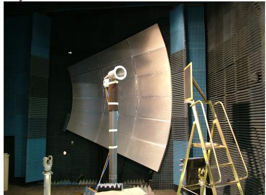
Fig. 4 X-band corrugated horn AUT installed within QMUL CATR shown together with 0.6 m by 0.6 m reflecting plate, shown to right of picture.
