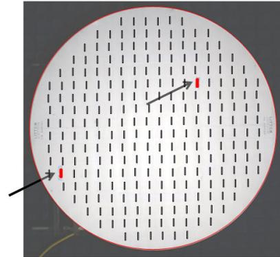
Fig. 1. Overlay of Element Map and Photograph of the 18 inch Flat Plate Array with the Blocked Elements Marked in Red
