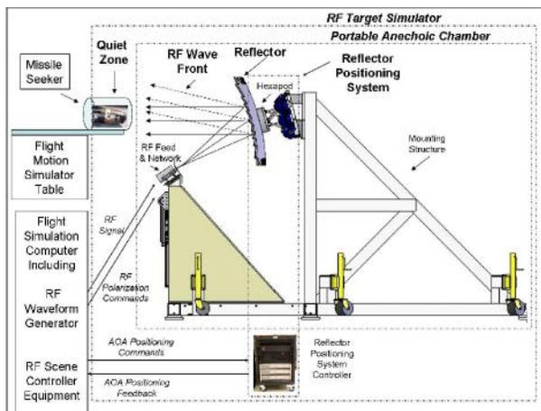
**Figure 1 RF Target Simulator Block Diagram**
