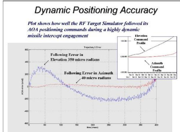
Figure 12 Dynamic Positioning Accuracy
