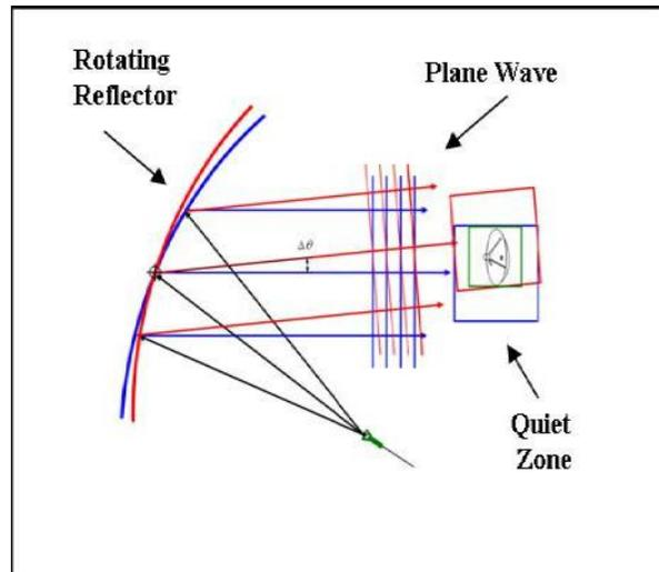
Figure 4 Rotated Reflector And Its Quiet Zone
