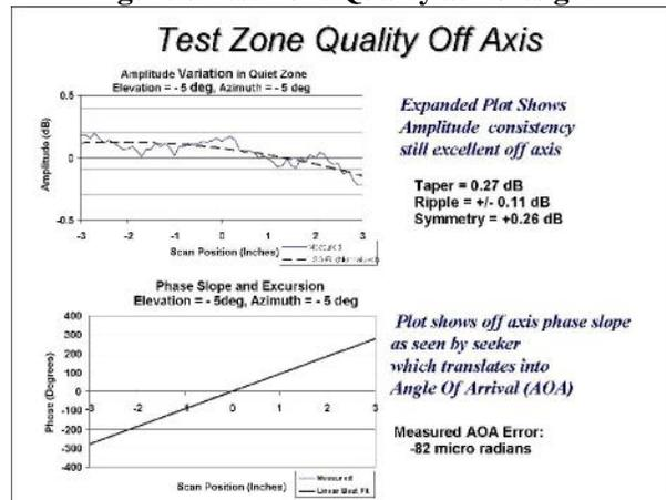
Figure 7 Test Zone Quality Off Axis
