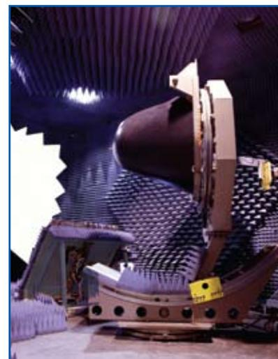
Figure 2: Radome testing in compact range system
