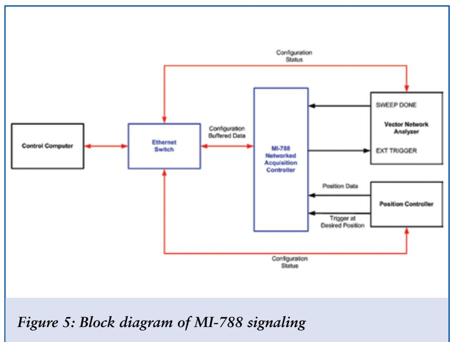
Figure 5: Block diagram of MI-788 signaling
