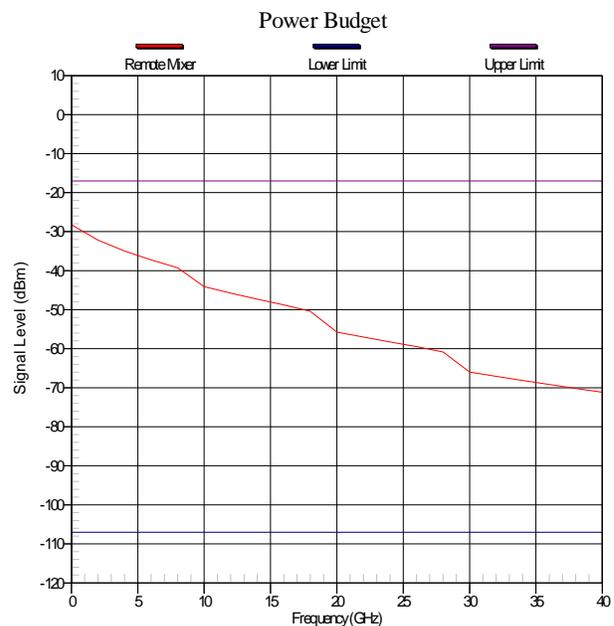
**Figure 4 Remote Mixer RF System Power Plot**
