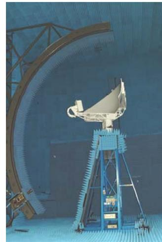
Fig.6. Photo of Arch with Reference Radar Antenna and Rotator for Evaluation of Test Facility
