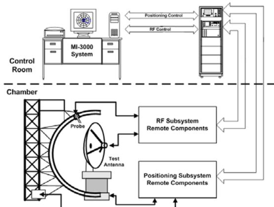
Fig.5. MI-3000 with Typical Spherical Near-Field Arch
