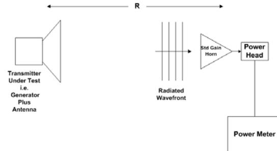
Fig 2. Schematic – Far-Field Measurement of EIRP received power.
