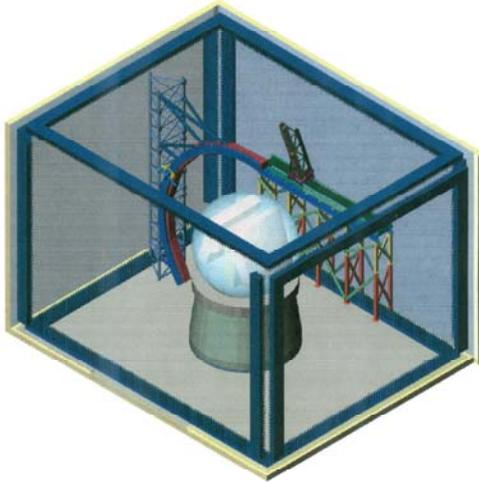
Fig.1. Schematic - Layout of the SAMPSON Radar Antenna Test Chamber
