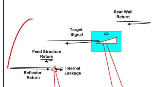
Fig. 9. Schematic- Some Sources of Radar Return in a Compact Range
