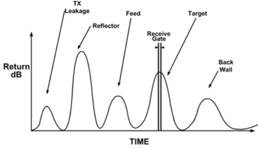
Fig. 8. Schematic Radar Return versus Time in a Compact Range
