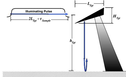
Fig. 11. Schematic – Rule for Height of Target Mount and Pylon
