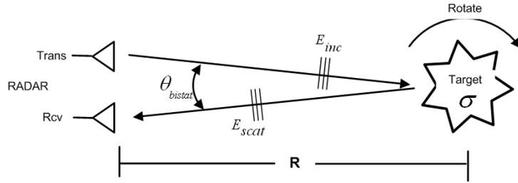
Fig. 1. Schematic of Bistatic Geometry for Measurement of Radar Cross Section
