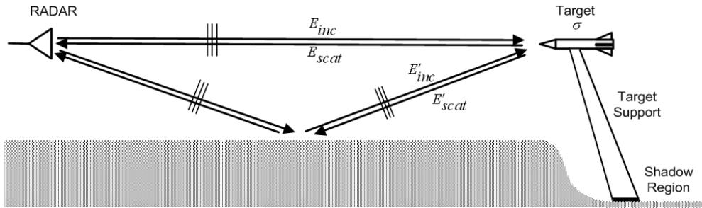
Fig. 2. Schematic of Ground Reflection Range with Shadow Region for Measurement of Ground-Based Radar Target
