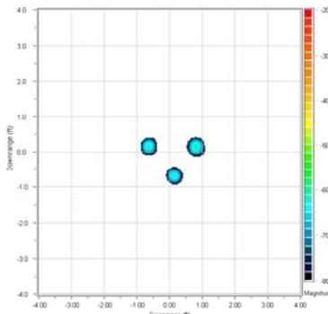
Fig.15. RCS Image of Three Spheres Each Having a  $-61$  dBsm Cross Section. Color Scale is  $-20$  to  $-80$  dBsm
