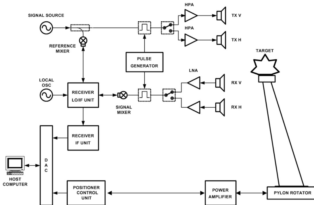
Fig. 13. Block Diagram of an Automated RCS Measurement System
