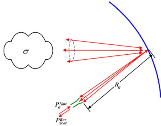
Fig. 7. Schematic of a Point Source Compact Range for RCS Measurement
