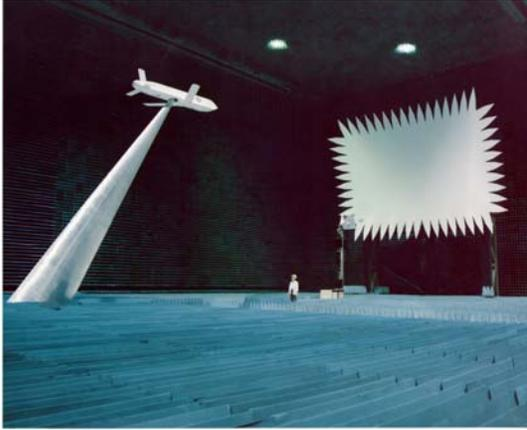
Fig. 6. Photo of a Point Source Compact Range for RCS Measurement
