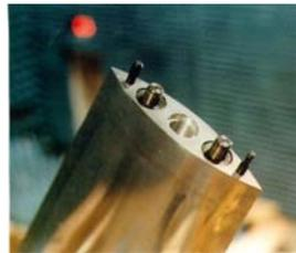
Fig. 4 Photo of Mounting Interface at the Top of the Pylon Base
