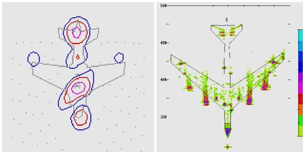
Fig.14. Example - Overlay of Two-Dimensional RCS Images with Envelope of Aircraft Outlines- Plan View
