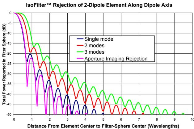
**Figure 18 - Comparison for 8.0 GHz - Plot of Image Level versus Distance Along x-Axis for Single Element at 8.0 GHz Together with *IsoFilter*<sup>TM</sup> Rejection Curves**
