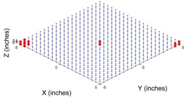
**Figure 11 - Schematic of 21 X 21 Element Sparse Array**
