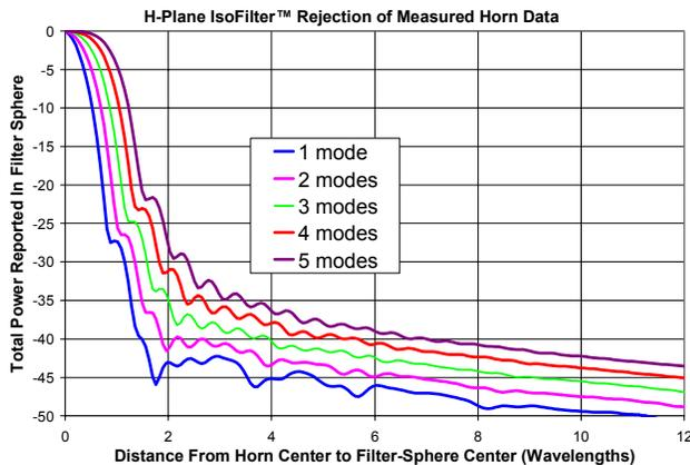
**Figure 6 - *IsoFilter*<sup>TM</sup> Rejection of Measured Horn Along x-Axis. Plot of Normalized Total Power versus Radial Distance of Filter Sphere from Center**
