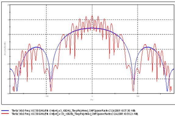
Figure 14 –Far Field of Sparse Array Before & After *IsoFilter*<sup>TM</sup> to Center Element
