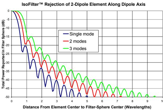
**Figure 9 - Rejection Curve for Two-Dipole Element *IsoFilter*™ with Origin Translated Along x-Axis**
