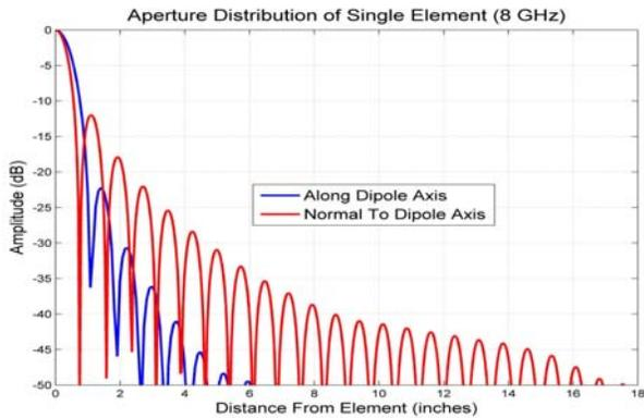
**Figure 17 - Plot of Image Level versus Distance for Single Element at 8.0 GHz**
