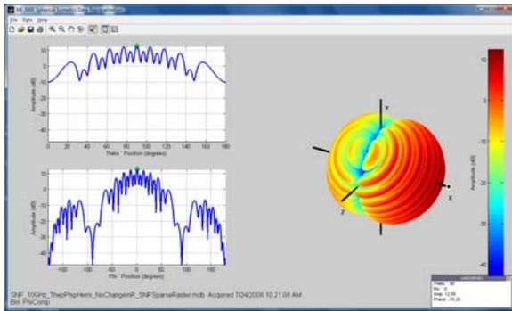
Figure 12 - Sparse Array's Far Field at 10.73 GHz.
