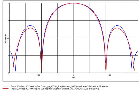
Figure 15 – Center-Element Far Field After *IsoFilter*<sup>TM</sup> vs. Actual Far Field of Ideal Element
