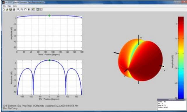
**Figure 8 - Two-Dipole Element Pattern ( $\phi$  Component)**
