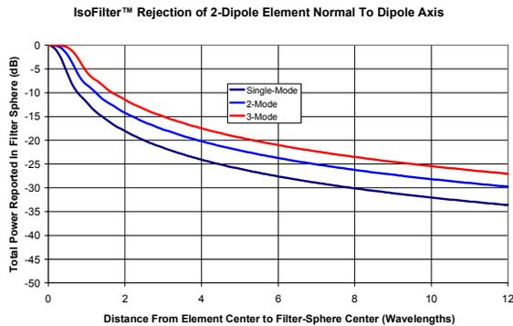
**Figure 10 - Rejection Curve for Two-Dipole Element *IsoFilter*™ with Origin Translated Along y-Axis or Along z-Axis**
