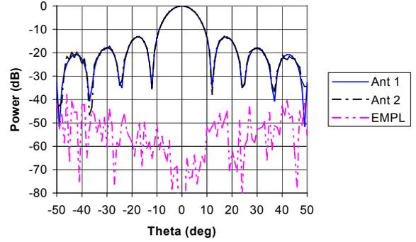
Figure 1. Cuts through Antenna patterns and EMPL.
