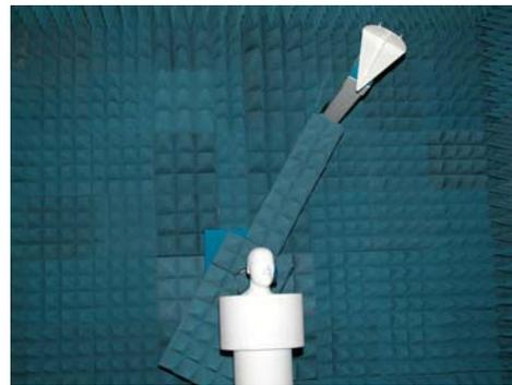
**Figure 13: Test with Phantom Head**
