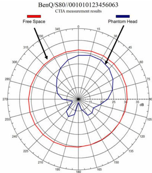
**Figure 9: Mobile Phone Radiation Patterns**
