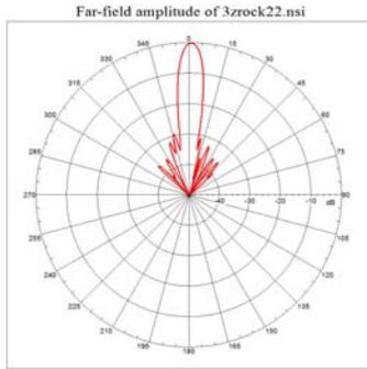
**Figure 2: High Gain Antenna Pattern**
