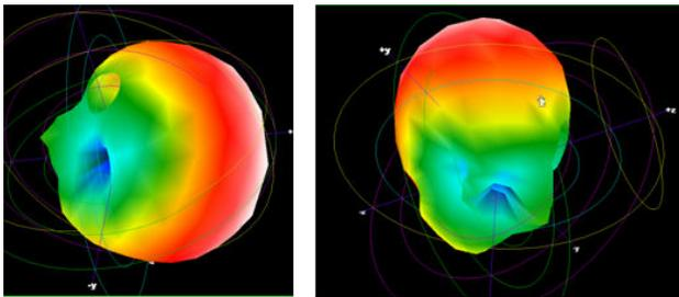
**Figure 14: 3D Radiation Patterns of Phone on Phantom Head**
