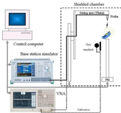
**Figure 5: 700S-90 OTA Test Set Up**
