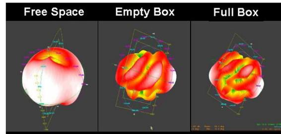
**Figure 10: RFID Tag 3D Radiation Patterns**
