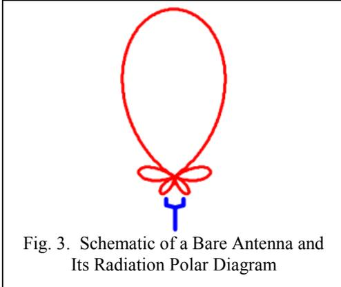
Fig. 3. Schematic of a Bare Antenna and Its Radiation Polar Diagram
