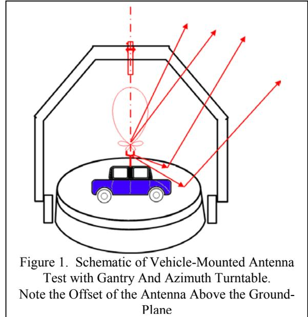
Figure 1. Schematic of Vehicle-Mounted Antenna Test with Gantry And Azimuth Turntable. Note the Offset of the Antenna Above the Ground Plane
