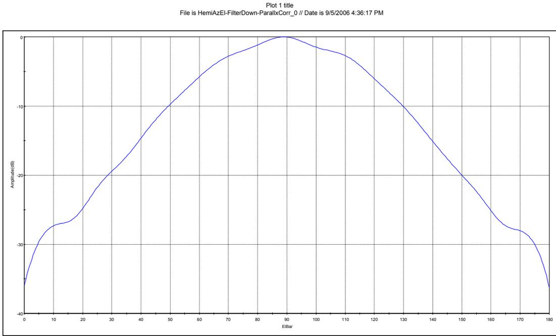
Figure 6a. *IsoFilter*<sup>TM</sup>ed Elevation Cut of Horn Mounted Near the Edge of a 36 inch Diameter Ground Plane
