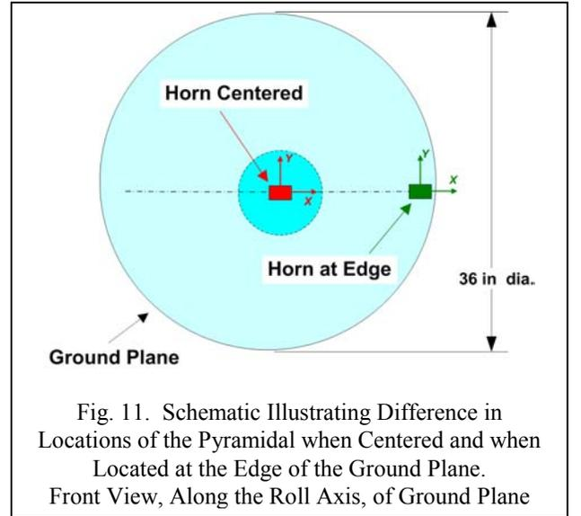
Fig. 11. Schematic Illustrating Difference in Locations of the Pyramidal when Centered and when Located at the Edge of the Ground Plane. Front View, Along the Roll Axis, of Ground Plane
