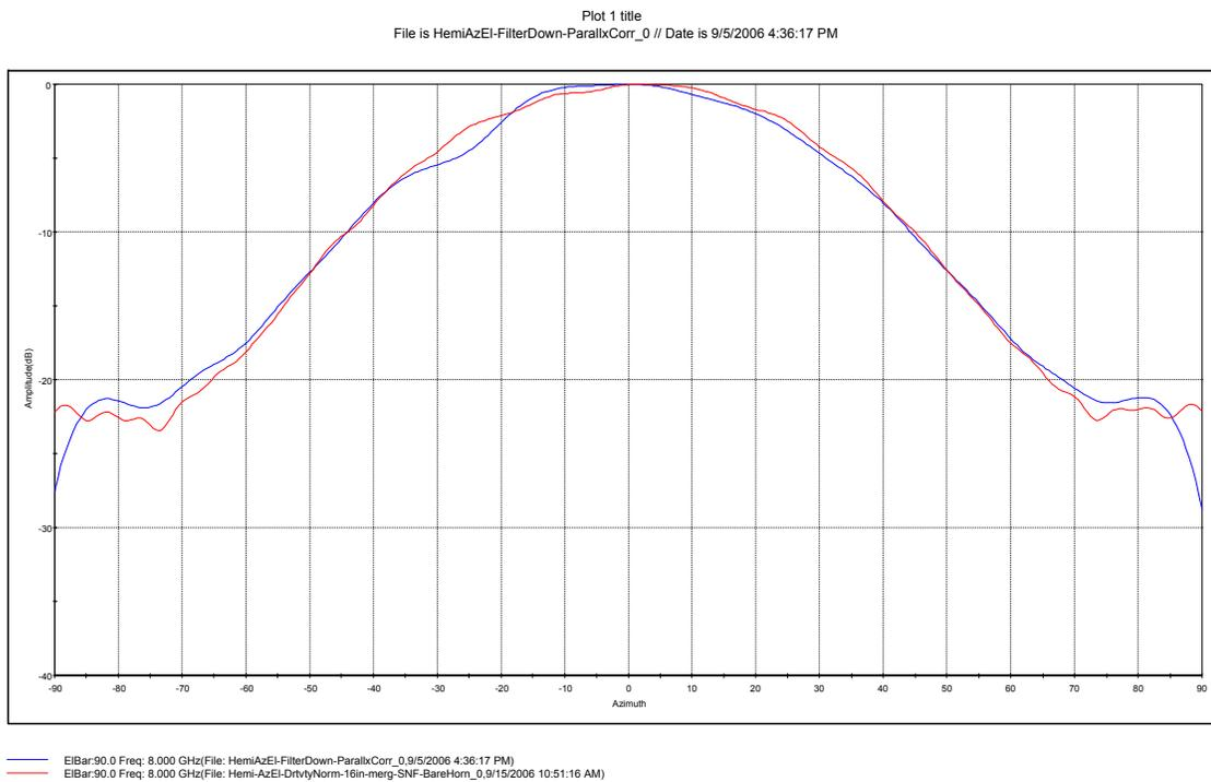
Figure 9b. *IsoFilter*<sup>™</sup>'ed Azimuth Cut of Horn Mounted Near the Edge of a 36 inch Diameter Ground Plane
