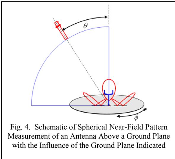
Fig. 4. Schematic of Spherical Near-Field Pattern Measurement of an Antenna Above a Ground Plane with the Influence of the Ground Plane Indicated
