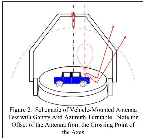
Figure 2. Schematic of Vehicle-Mounted Antenna Test with Gantry And Azimuth Turntable. Note the Offset of the Antenna from the Crossing Point of the Axes
