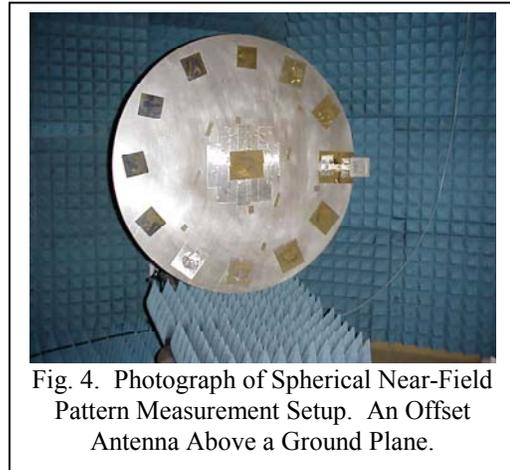
Fig. 4. Photograph of Spherical Near-Field Pattern Measurement Setup. An Offset Antenna Above a Ground Plane.
