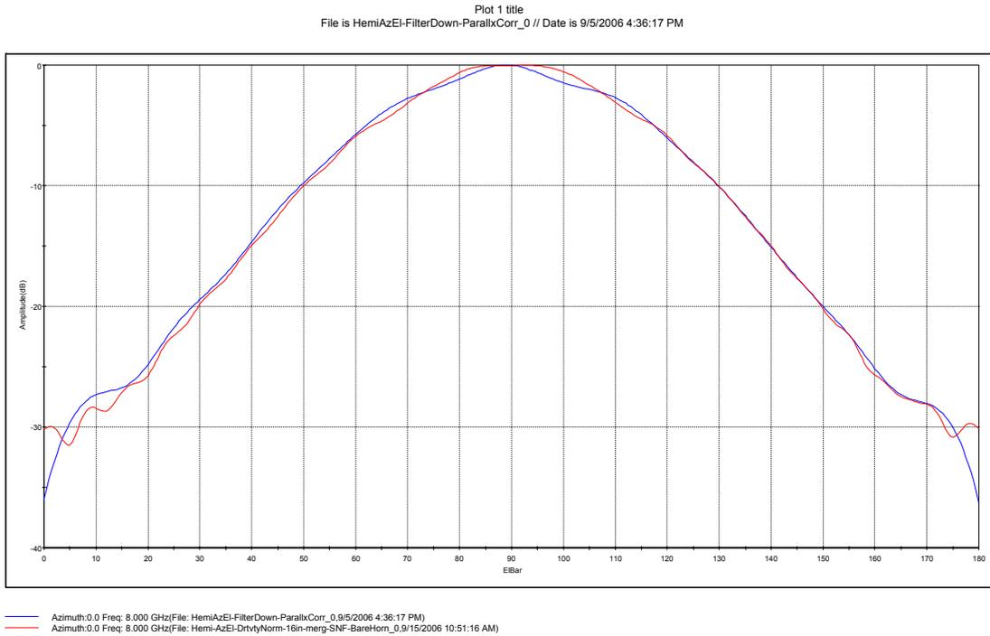
Figure 9a. *IsoFilter*<sup>™</sup>'ed Elevation Cut of Horn Mounted Near the Edge of a 36 inch Diameter Ground Plane
