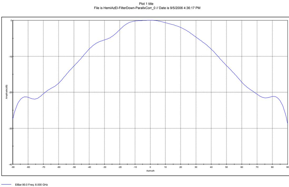
Figure 6b. *IsoFilter*<sup>TM</sup>ed Azimuth Cut of Horn Mounted Near the Edge of a 36 inch Diameter Ground Plane
