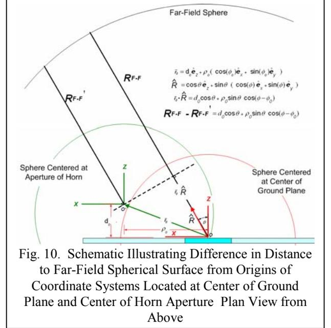
Fig. 10. Schematic Illustrating Difference in Distance to Far-Field Spherical Surface from Origins of Coordinate Systems Located at Center of Ground Plane and Center of Horn Aperture. Plan View from Above
