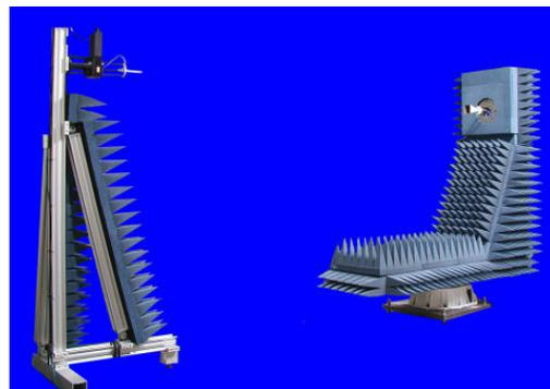
Figure 3 – NSI-700S-60 SNF scanner used in the testing
