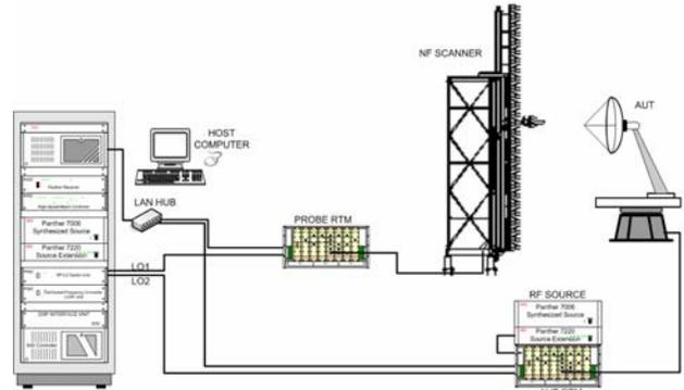
**Figure 4 –System Block Diagram using RTMs**
