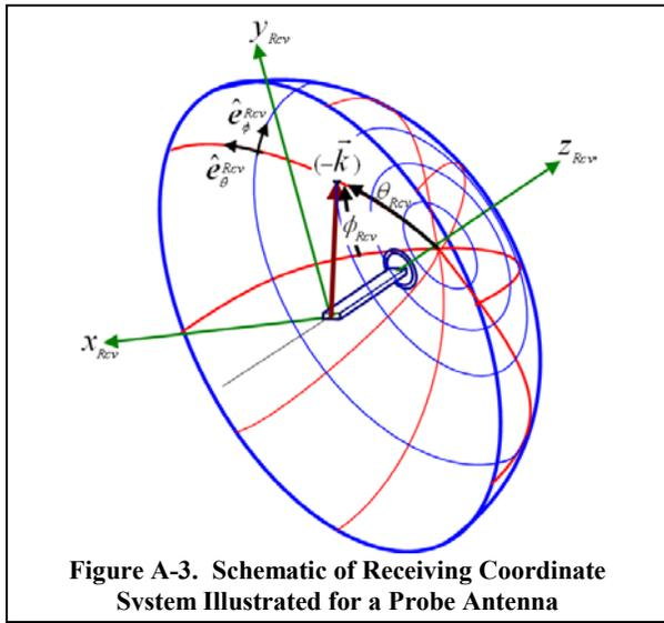
Figure A-3. Schematic of Receiving Coordinate System Illustrated for a Probe Antenna
