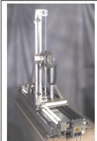
**Fig.5, An x-y Positioner Used as Null Seeker**
