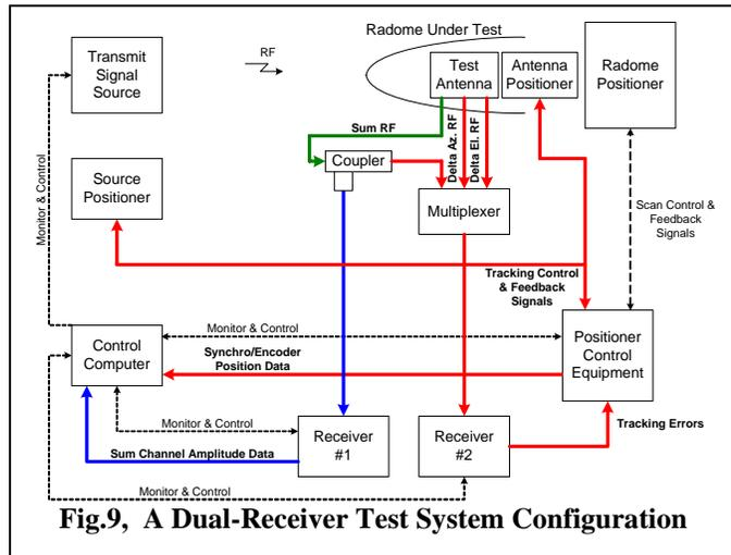
**Fig.9, A Dual-Receiver Test System Configuration**
