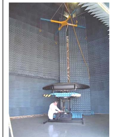
**Fig.14, A 6 m Cylindrical NF Range**
