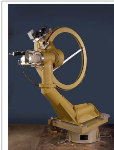
**Fig.7, Three-Axis Radome Positioner**
