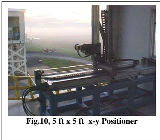
**Fig.10, 5 ft x 5 ft x-y Positioner**
