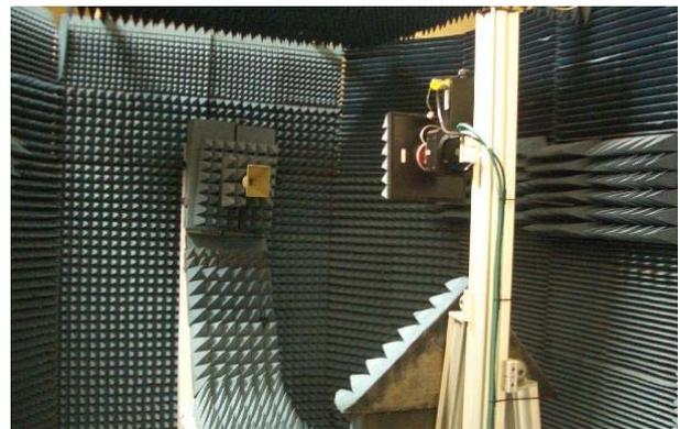
Figure 2 – NSI-700S-60 Spherical NF Test Range
