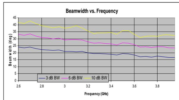
Figure 18 –Beamwidth versus frequency on 700S-90 scanner – no absorber or chamber – WITH MARS
