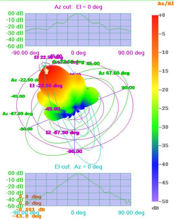
Figure 6 – NSI-RF-SG284 Standard Gain Horn tested on NSI-700S-90 scanner with no absorber or chamber – MARS correction OFF
