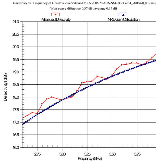
**Figure 14 – Directivity vs. frequency on 700S-60 in chamber at NSI, compared to NRL directivity**
