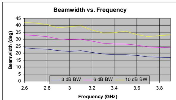
Figure 16 –Beamwidth versus freq - 700S-50 chamber
