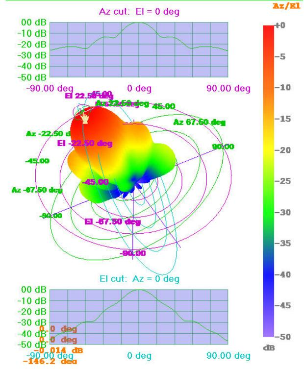
Figure 7 – NSI-RF-SG284 Standard Gain Horn tested on NSI-700S-90 scanner with no absorber or chamber – MARS correction enabled
