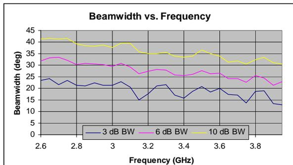
Figure 17 –Beamwidth versus frequency on 700S-90 scanner – no absorber or chamber
