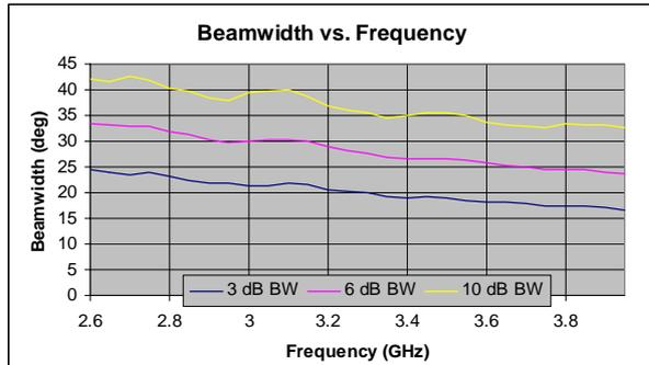
Figure 15 –Beamwidth versus freq - 700S-60 chamber
