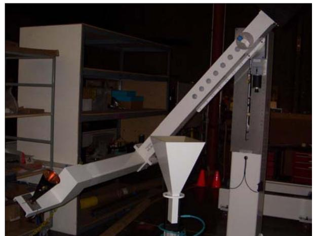
Figure 3 – NSI-700S-90 Spherical NF Test Range
