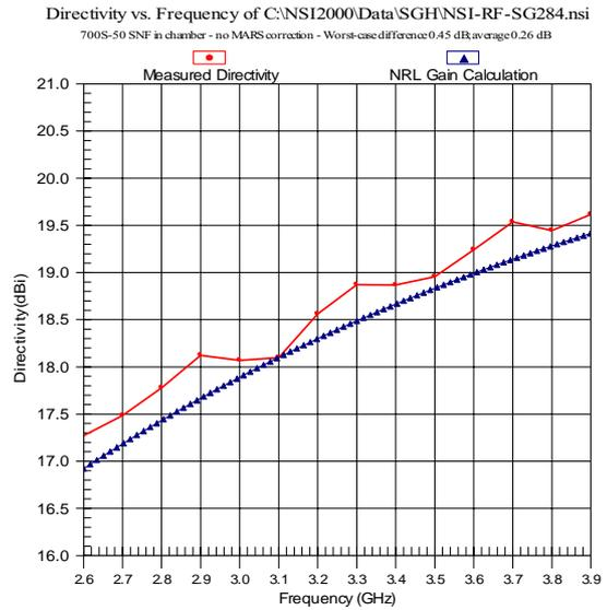
**Figure 13 – Directivity vs. frequency on 700S-50 in chamber at customer site, compared to NRL directivity (only 14 frequencies)**
