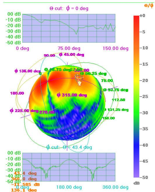
**Figure 4 – NSI-RF-SG284 gain horn tested at NSI on NSI-700S-90 ARCH Spherical NF in open environment with NO anechoic chamber – notice ripple in pattern at about -25 dB level due to range reflections**
