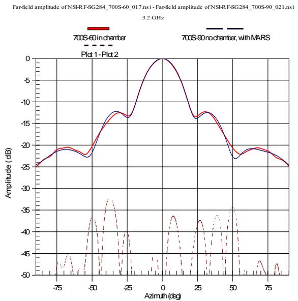
**Figure 10 – Far-field comparison at 3.20 GHz of SGH data taken in chamber versus on 700S-90 ARCH range with no absorber or chamber, with MARS correction enabled**
