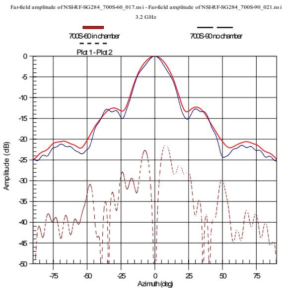
**Figure 9 – Far-field comparison at 3.20 GHz of SGH data taken in chamber versus on 700S-90 ARCH range with no absorber or chamber, with no MARS correction**
