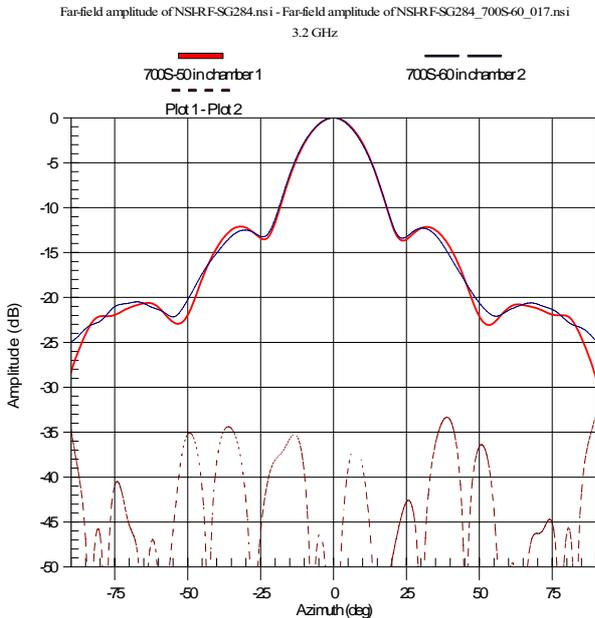
**Figure 8 – Far-field comparison at 3.2 GHz of SGH data taken in NSI chamber vs. customer chamber**
