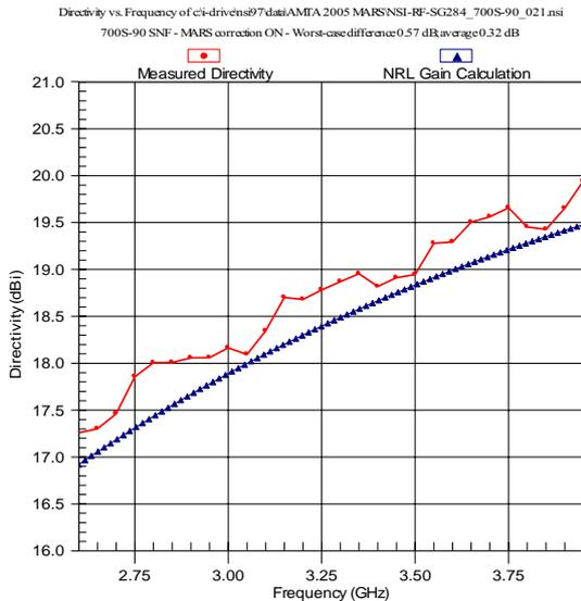
**Figure 12 – Directivity versus frequency on 700S-90 ARCH range with no absorber or chamber, compared to NRL directivity, with MARS correction**
