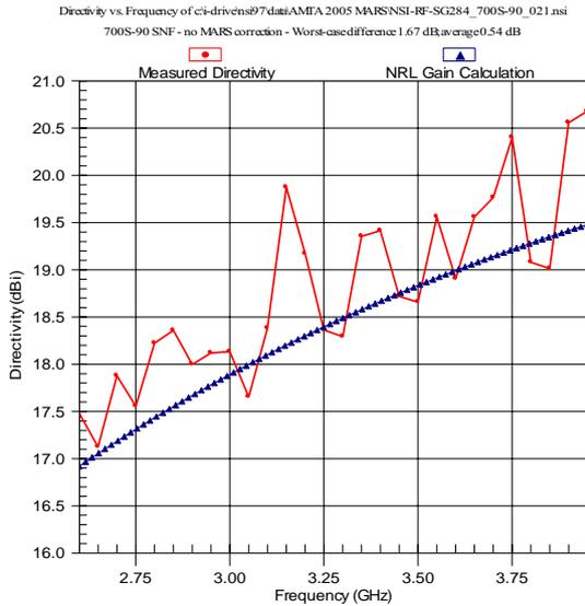
**Figure 11 – Directivity vs. frequency on 700S-90 ARCH range with no absorber or chamber, compared to NRL directivity, with no MARS correction**
