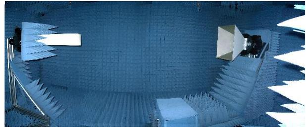
Figure 1 – NSI-700S-50 Spherical NF Test Range
