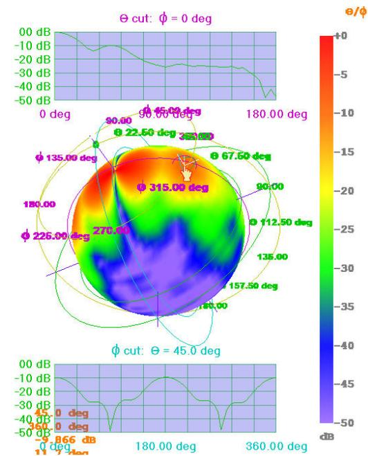
**Figure 5 – NSI-RF-SG284 gain horn tested at NSI on NSI-700S-60 Spherical NF in chamber**
