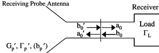
**Figure 5 - At the Receiving Antenna - Range in “Range-Inserted” Configuration**
