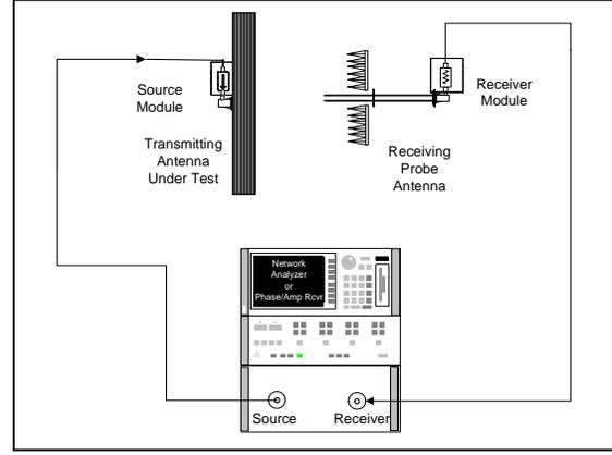
Figure 2 - Schematic of Planar Near-Field Range with AUT in Transmit as Set Up for Measurement of the Received Phasor  $b_0'$ .
