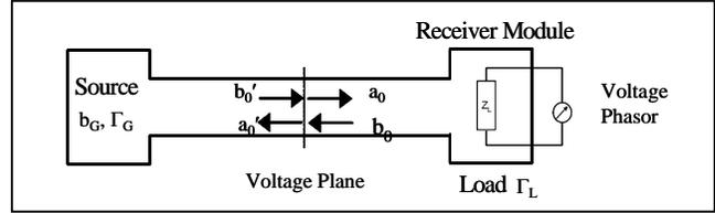
Figure A1 – Circuit Model of a Voltage Receiver
