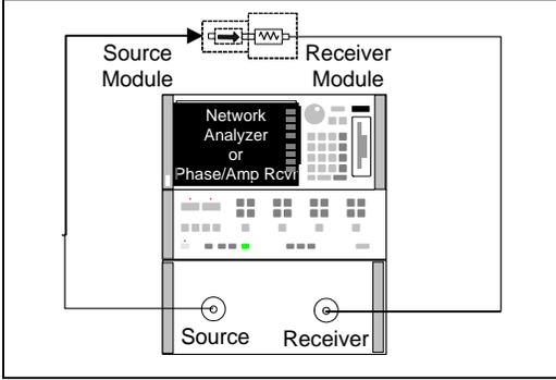
Figure 1 - Range in "Through" or "Short Circuited" Condition for Measurement of Incident Phasor  $a_0$ .
