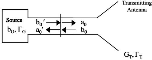
**Figure 4 - At the Transmitting Antenna - Range in “Range-Inserted” Configuration**
