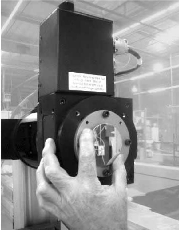
**Figure 9 – Using Front Surface Mirror to Determine Axis Alignment**
