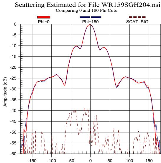
Figure 4 – Near-field scattering test checking chamber sidewalls
