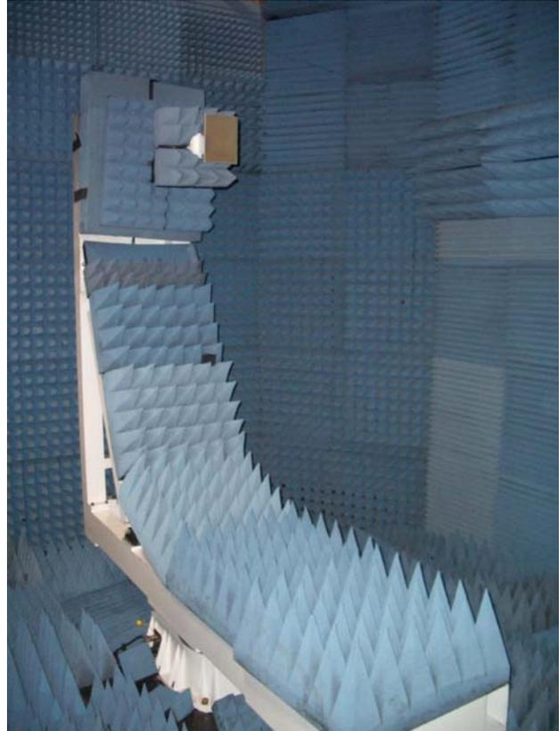
**Figure 1 – NSI 700S-60 Spherical Near-field Scanner shown testing a WR-159 Standard Gain Horn**
