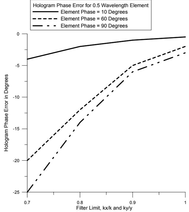
**Figure 5 Hologram phase error for 0.5 wavelength element for typical filter limits.**
