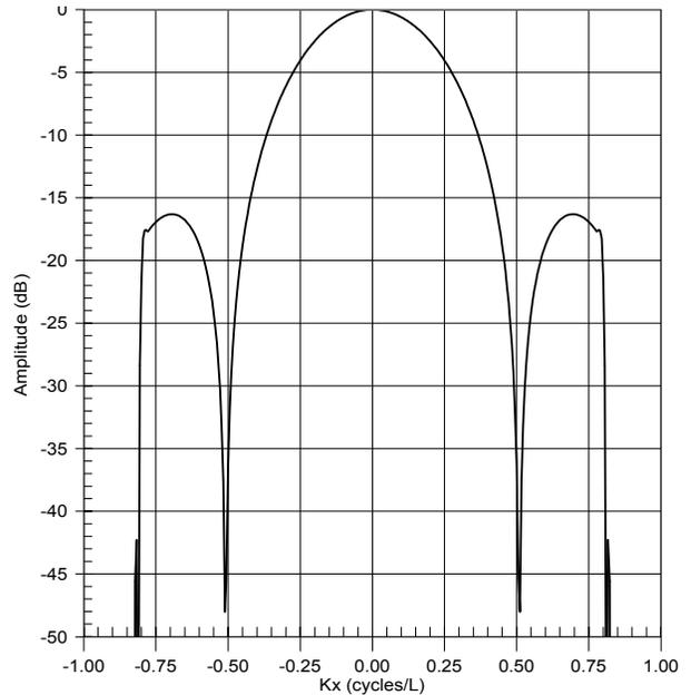
**Figure 3 Spectrum of square wave filtered to  $k_x = 0.8$ .**
