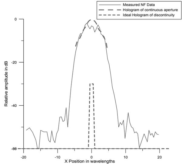
**Figure 1 Example of measured near-field data and the two parts of the hologram**
