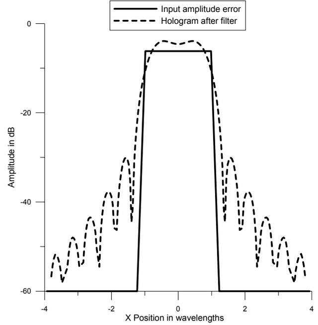
**Figure 2 Example of amplitude error pulse and calculated hologram with filter at  $k_x = k_y = 1.0$ .**
