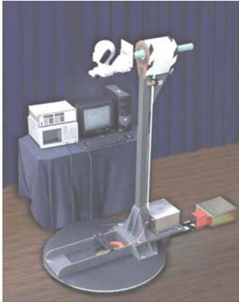
Figure 3. Two-axis dielectric positioner
