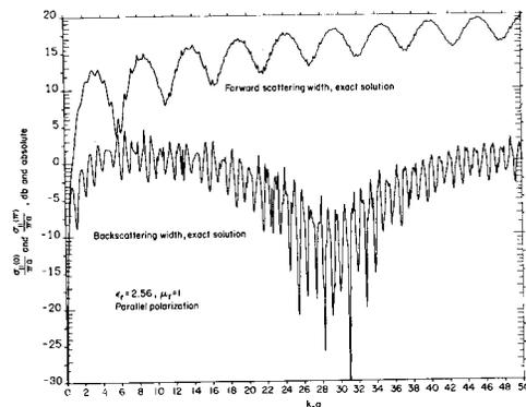
Figure 2. Backscatter and forward scatter from an infinitely long, lossless homogeneous dielectric cylinder at normal incidence for parallel polarization.
