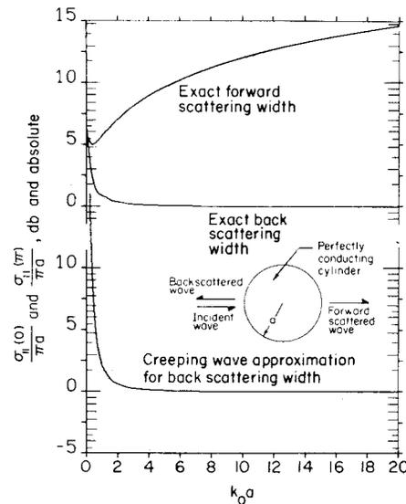
Figure 1. Backscatter and forward scatter from an infinitely long, perfectly conducting circular cylinder at normal incidence for parallel polarization.
