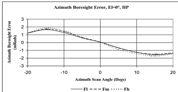
**Figure 7:** Azimuth Boresight Error vs. Azimuth Scan Angle- Horizontal Polarization.
