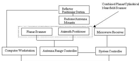
**Figure 3:** Simplified System Block Diagram
