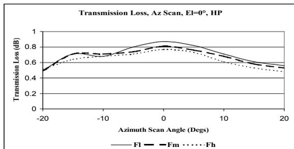
**Figure 5:** Transmission Loss vs. Azimuth Look Angle- Horizontal Polarization.
