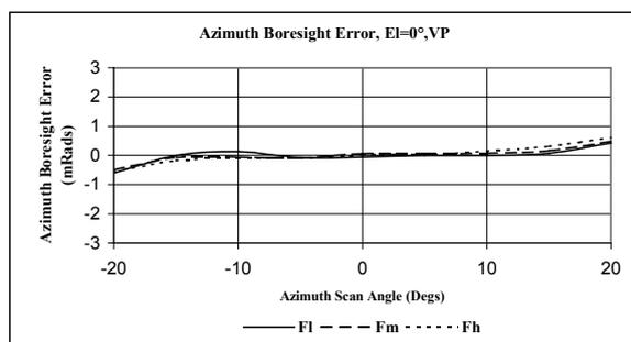
**Figure 8:** Azimuth Boresight Error vs. Azimuth Scan Angle- Vertical Polarization.
