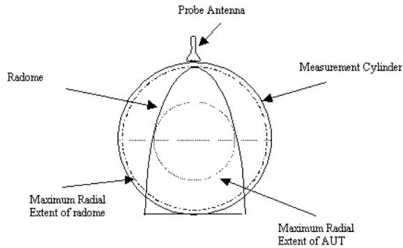
**Figure 4: Radome/Measurement Cylinder Geometry**
