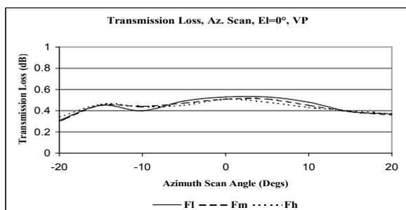
**Figure 6:** Transmission Loss vs. Azimuth Look Angle- Vertical Polarization.
