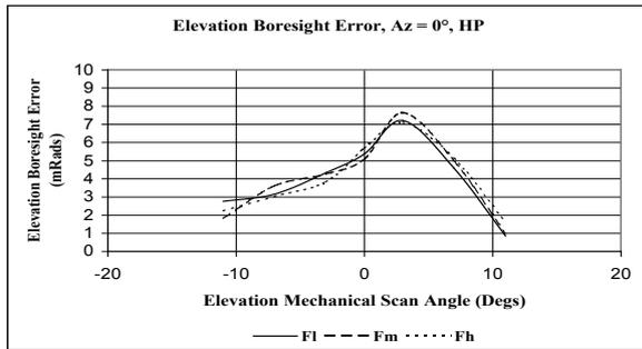
**Figure 9:** Elevation Boresight Error vs. Mechanical Reflector Angle, Horizontal Polarization.
