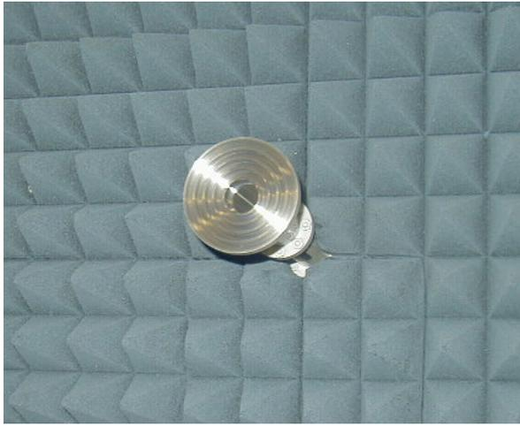
**Figure 2:** Probe antenna aperture.
