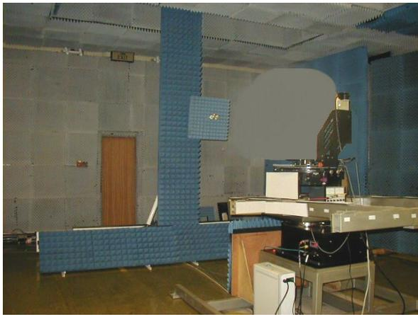
**Figure 1:** Combined Planar/Cylindrical Scanner.
