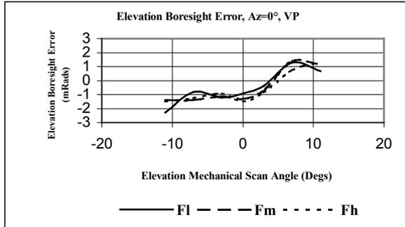
**Figure 10:** Elevation Boresight Error vs. Mechanical Reflector Angle, Vertical Polarization.
